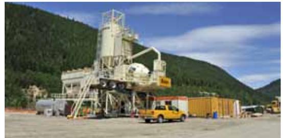
Mica batch plant that will produce concrete needed for installation of new generating units.
