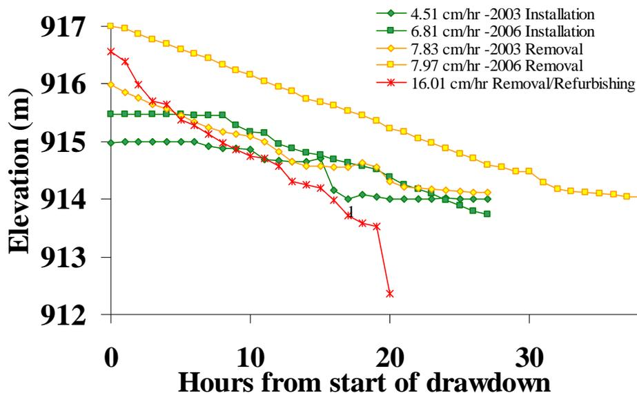
**Figure 3.** Headpond elevation (m) versus hours from start of (hr). Green, yellow and red lines indicate removal (April/May) and installation of flashboards (July) and refurbishing/removal (July 2005), respectively.
