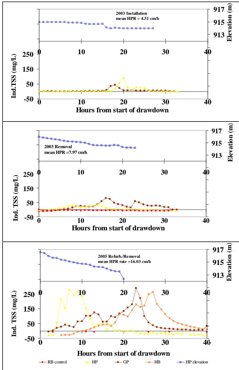
**Figure 4.** Induced TSS (mg/L) and headpond elevation (m) as a function of time from the start of for example operations. HPR = headpond reduction rate. See Figure 2 and Table 1 for locations and descriptions of sites.
