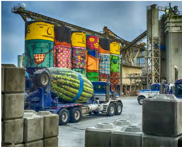
Concrete is usually delivered within about an hour of 'batching', which is when water is added at the concrete plant
