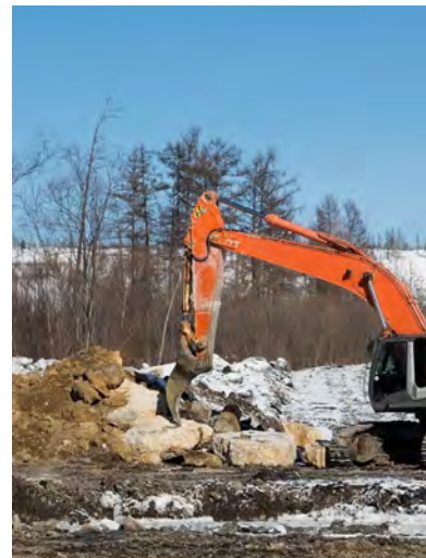
Example excavator with ripping-tooth attachment
