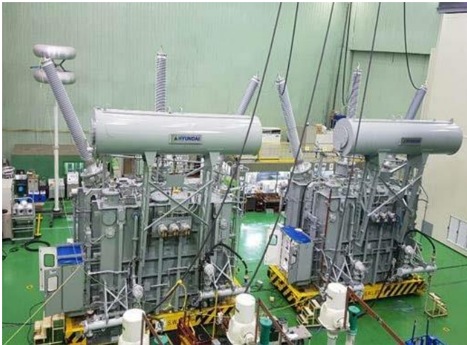
Transformers 7 and 8 under factory testing at the manufacturer's facility
