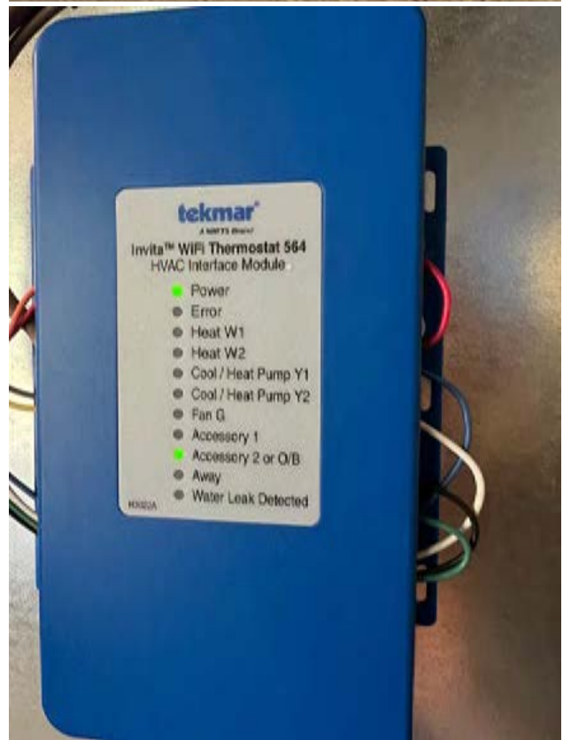
Figure 9 Examples of Controllers; Tstat Wiring (top) and Sample Controller that can Manage Multiple Units (bottom)
