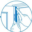
Use door weatherstripping and outlet and switch gaskets to reduce drafts
