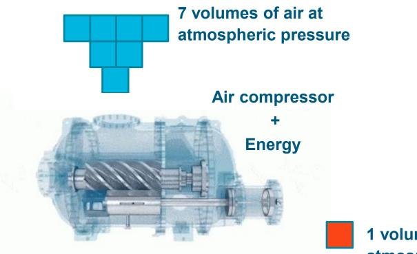
1 volume of air at 7x atmospheric pressure
