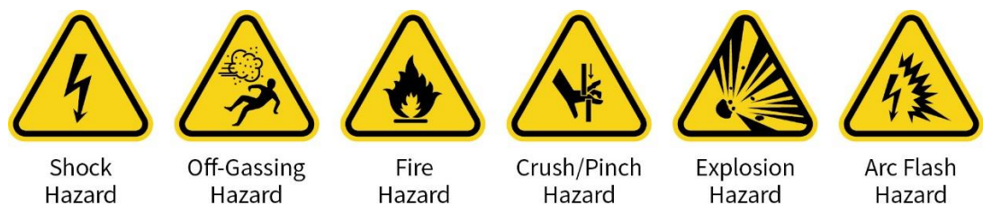
Figure 11-1: Common Hazard Labels Associated with BESS
