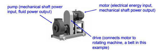
Pumps are part of some industrial process **systems**. What is a system? A system includes pumps and the associated equipment that all work together to do something useful such as deliver water for a cooling system, circulate refrigerant in a refrigeration system or pump sewage in a treatment system.
