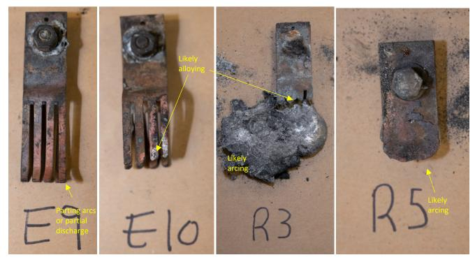
Figure 43: Contact forks found in debris underneath switch (left two), and debris south of switch (right two).
