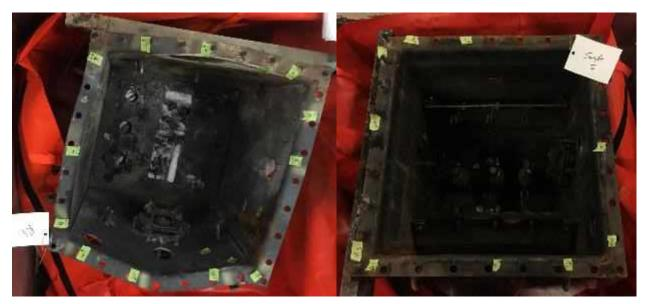
Figure 19. Locations on Switch 2019 and Switch 2018 subjected to Leeb hardness testing
