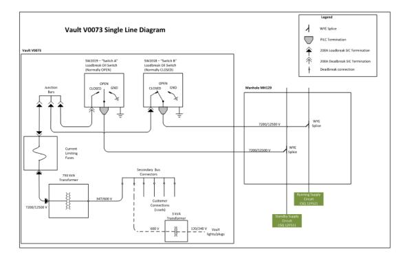
Figure 6: Vault V0073 Single Line Diagram.
