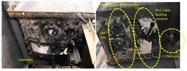
Figure 39: SW2019 underside of housing showing bowing (left), and absence of service connections (right).
