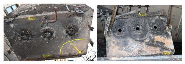
Figure 26: Bottom of CLF cabinet showing broken cables (left); top of CLF cabinet (right).
