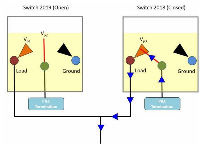
Figure 29. Arrangement of switches in vault 073 (Blue arrows indicate current flow)
