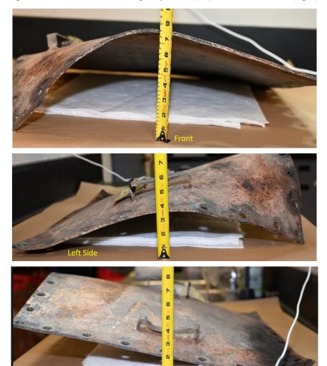
Figure 37: SW2019 lid deformation, observed during a laboratory examination.
