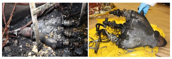
Figure 40: SW2019 PILC Connector and Termination as found (left); in laboratory (right).
