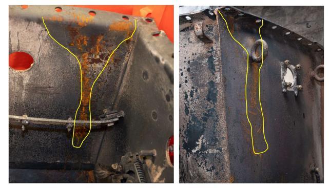
Figure 57: Corrosion region on inside and outside of the switch housing aligning with three bolt openings.
