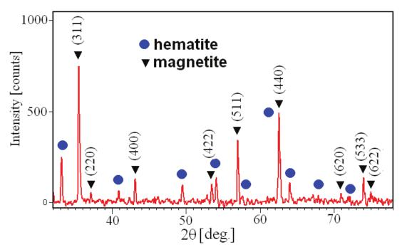
Figure 18. Reference XRD patterns for hematite and magnetite
