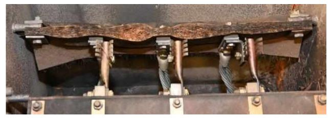
Figure 11. Insulating bar from switch 2018 showing expansion due to be being exposed to high external heat
