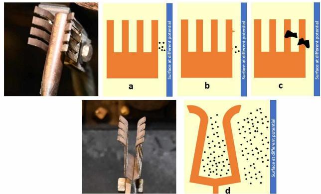
Figure 30. Sketches of scenarios that would lead to PD or arcing at contacts (not to scale)
