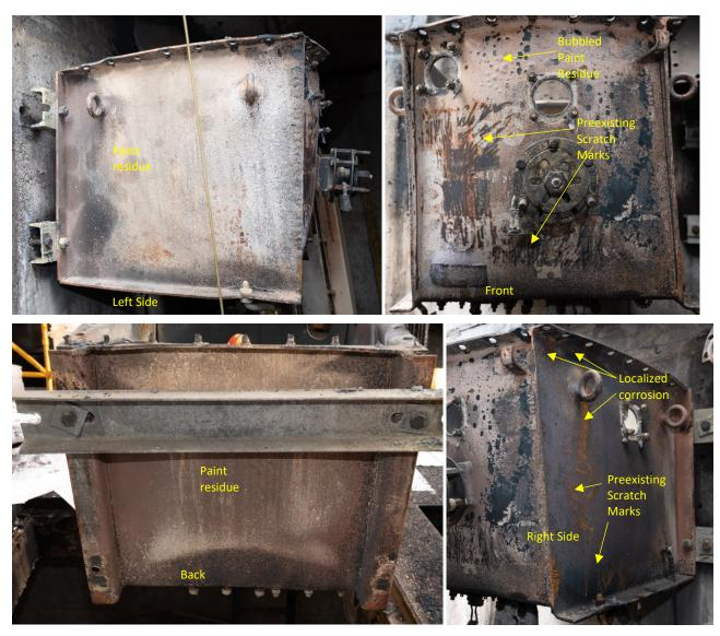
Figure 34: Images showing the perimeter faces of the SW2019 housing.
