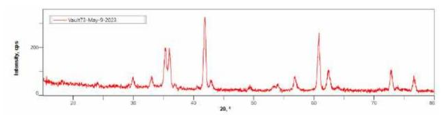
Figure 17. XRD pattern of the collected rust sample from switch 2019
