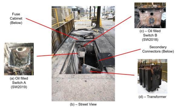
Figure 5: Vault V0073 Layout after the explosion.
