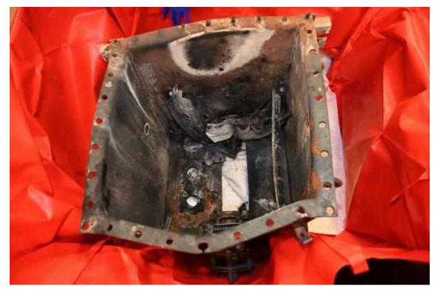
Figure 2. Top down view into switch 2019 (as received)
