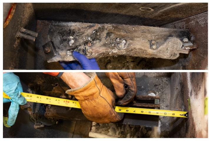
**Figure 53:** Service insulating board assembly showing gap at left side (top); supply insulating board from SW2018 positioned in SW2019 showing gap due to deformation of the SW2019 housing.
