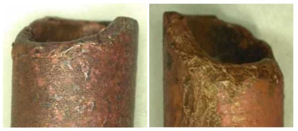
Figure 31. Microscope photos of two different example tips of copper blades from switch 2019
