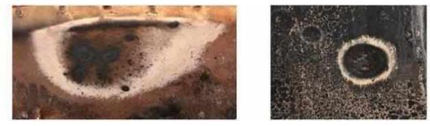
Figure 5. Close up of white rings on inside of the switch 2019 tank
