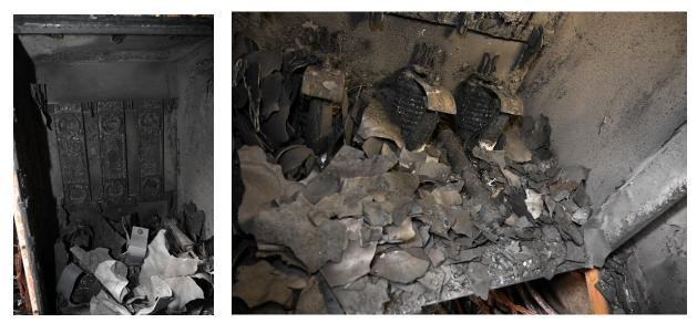
Figure 27: CLF cabinet inside (left); fuses and components found in debris at bottom (right).
