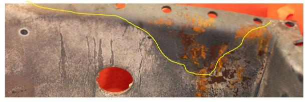
Figure 58: Region where no epoxy-enameled paint remained post-Incident.
