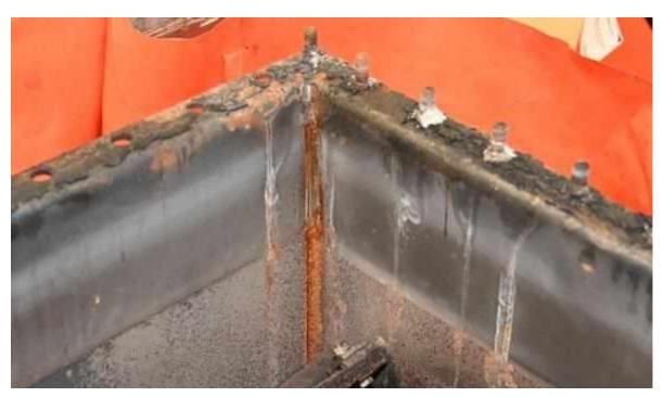
Figure 9. Close up of orange-brown residue on walls of switch 2018
