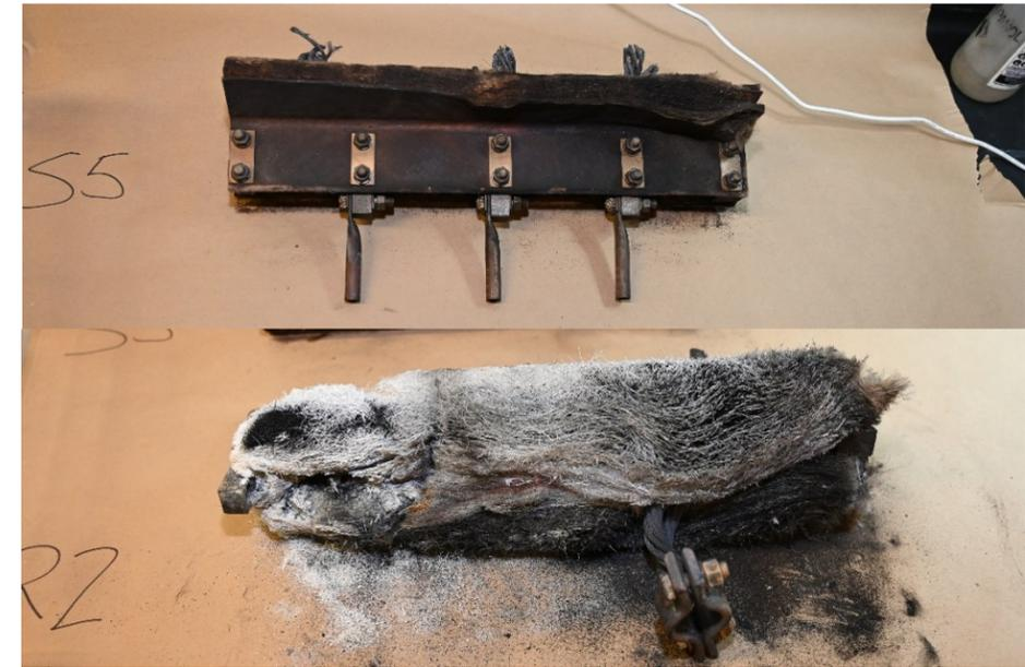
Figure 54: Insulation for Switch Hinge Pins (a) Switch 2018 (Sample S5); (b) Switch 2019 (Sample R2).
