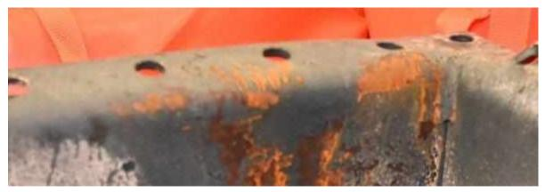
Figure 24. Damage at edge of tank right front
