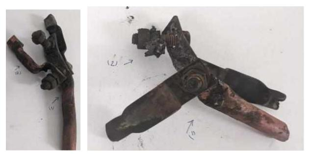
Figure 14. Blade assemblies analyzed from switch 2019
