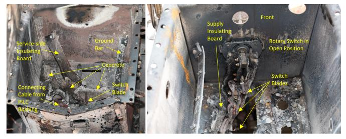
Figure 41: Interior of switch immediately post-incident (left); image of the front face of the switch box post-removal (right).
