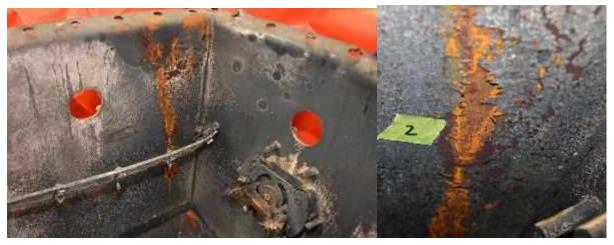
Figure 6. Close up photos of orange-brown areas inside of switch 2019 tank
