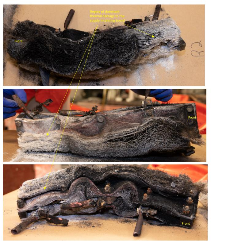
Figure 46: Images showing different views of supply insulating board with remaining blades and greater damage to the board at the back of the switch.
