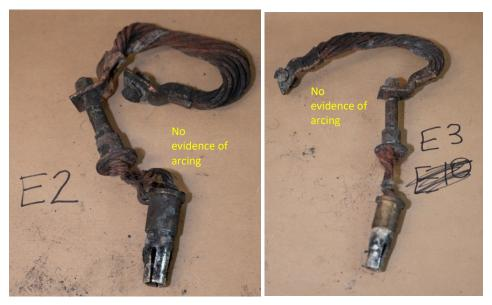
Figure 44: Elbow connector cables found in debris immediately below SW2019.
