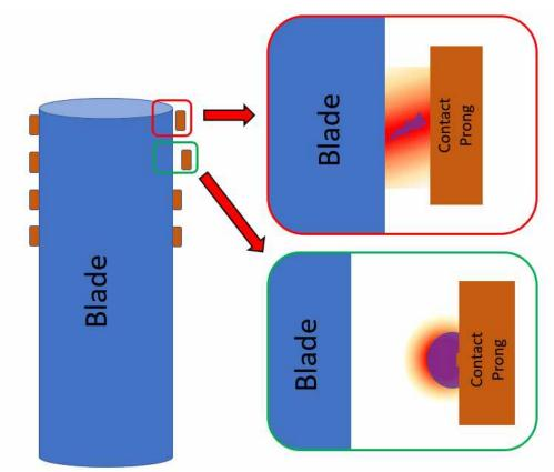
Figure 27. Diagram on the generation of PD or arcing at contact blades in switches Top: arcing; Bottom: PD
