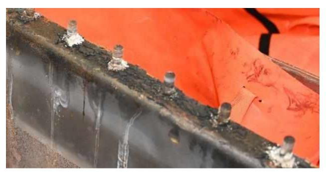
Figure 12. Close up of a region of carbonized and damaged gasket of switch 2018
