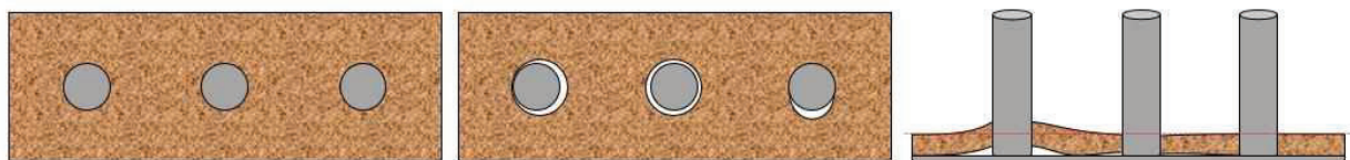
Figure 22. Diagram of possible holes made for gasket material Left: Good bolt interface; Middle: Too big of holes; Right: Gasket hole made too small
