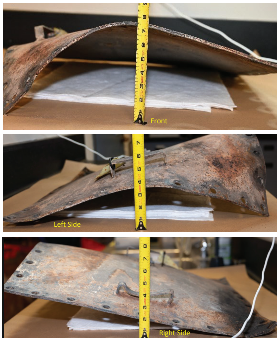
Figure 37: SW2019 lid deformation, observed during a laboratory examination.
