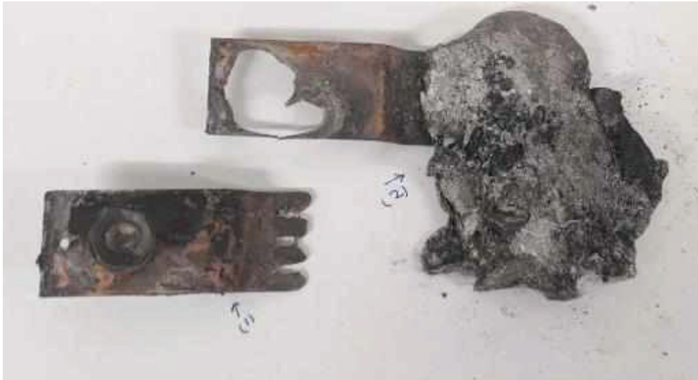
Figure 16. Selected contacts analyzed by SEM-EDS for elemental analysis Left: Bare Contact; Right: Contact with metallic mass at the end
