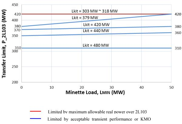
RTA to BCH Transfer limit Under system normal condition with 7 units at KMO and 4 capacitor banks at KIT
