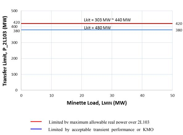
RTA to BCH Transfer limit Under system normal condition with 8 units at KMO and 4 capacitor banks at KIT
