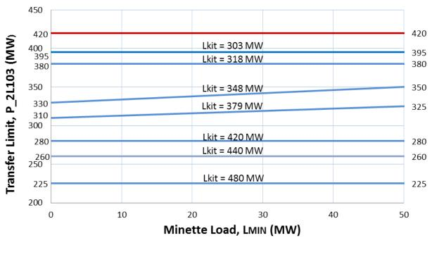
RTA to BCH Transfer limit Under system normal condition with 6 units at KMO and 4 capacitor banks at KIT
