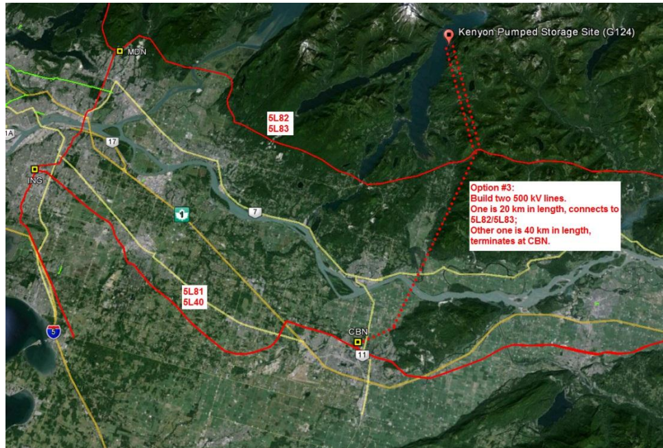
Figure 9 (c), Interconnection Option 3 for the new Lower Mainland Pumped Storage Generating Station
