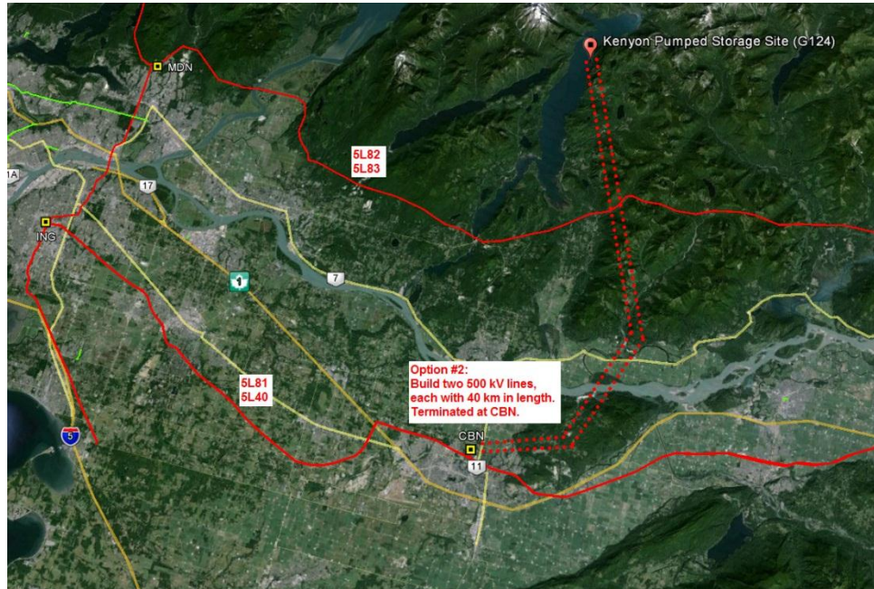
Figure 9 (b), Interconnection Option 2 for the new Lower Mainland Pumped Storage Generating Station.
