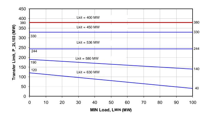
Limited by maximum allowable real power over 2L103 Limited by acceptable transient performance or KMO reactive power reserves
