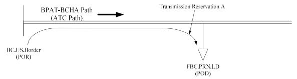
Transfer capability for the radial line connecting FBC.PRN.LD and the system has been planned and constructed to meet the peak load. Transmission Reservation A from BC.US.Border to FBC.PRN.LD impacts ATC on the BPAT-BCHA Path, and is counted as ETC when calculating ATC for this ATC Path. Such and similar transmission reservations are tracked, and used for calculating ATC by BC Hydro MODS, an OATI hosted system.
