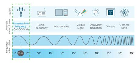
This diagram shows the different levels of energy that make up the electromagnetic spectrum. The energy of waveforms increases exponentially as the frequency moves from low to high.
