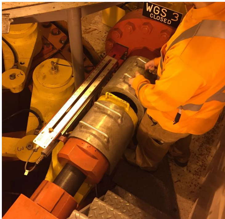
Figure 8. Worker applying mechanical blocking (horseshoe) to hydraulic cylinder
