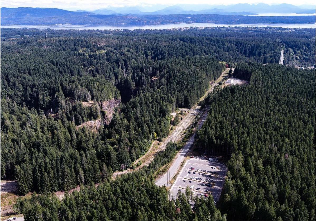
**Figure A-4 Completed Main and Service Portal Entrances, Remaining Surge Tower, and New Tailrace Area**
