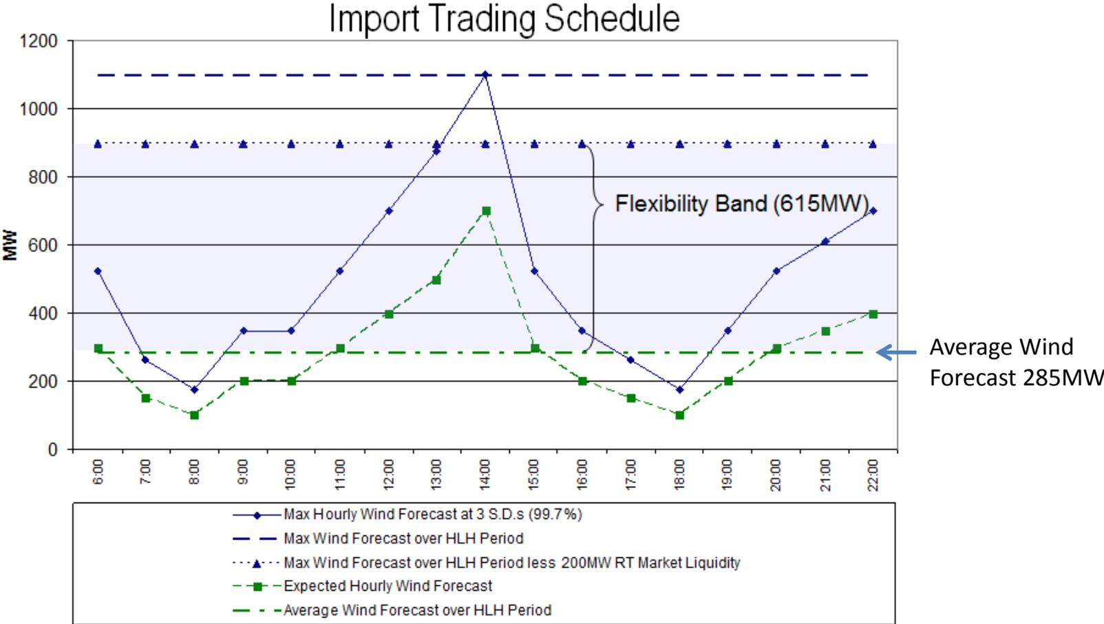
$$WOC = (615MW * (\$40/MWh (rsys) - \$10/MWh (Market Price)) * 16hrs) / (285MW * 16hrs) = \$64.74/MWh$$
