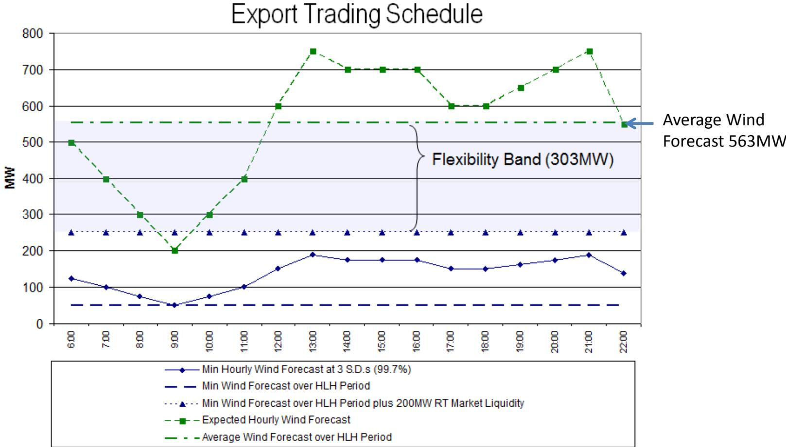
$$WOC = (303MW * (\$60/MWh \text{ (Market Price)} - \$40/MWh \text{ (rsys)}) * 16hrs) / (563MW * 16hrs) = \$10.76/MWh$$
