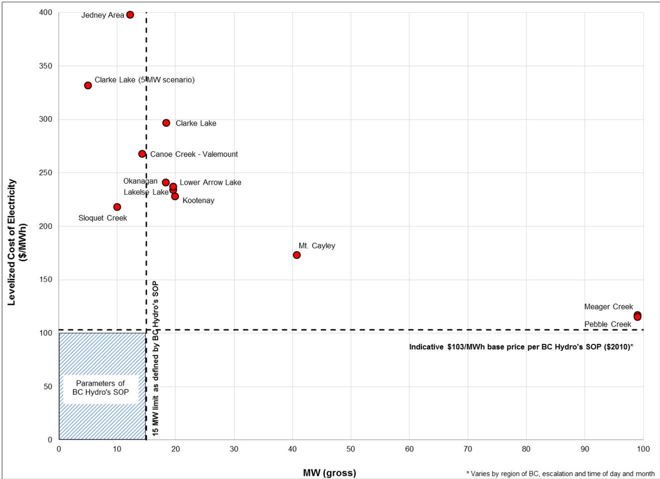
**Figure 7-2: Geothermal Sites – LCOE vs Capacity**
