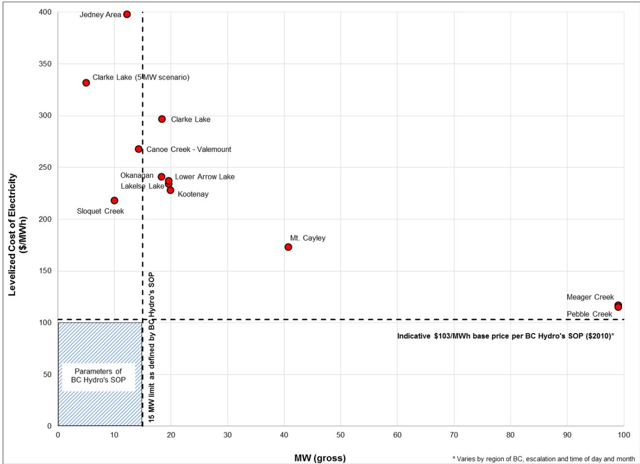
**Figure E1-3: Geothermal Sites – LCOE vs Capacity**
