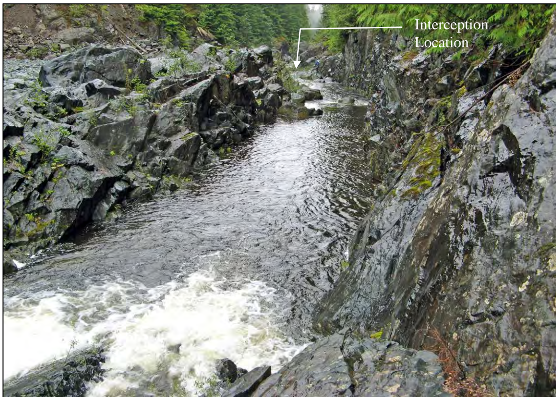
Photo 6. M2 salt dilution gauging section (looking downstream). Salt is released in the cascade and intercepted by the conductivity meter at the arrow. Photo taken Aug. 27, 2008; gauged flow 0.925 \text{ m}^3/\text{s} .
