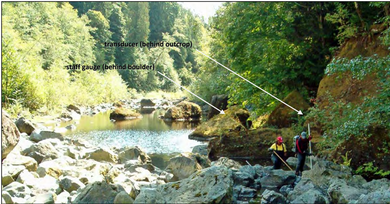
Photo 1. View of the M1 water level monitoring pool (looking downstream). The transducer was located on the right bank behind the bedrock outcrop; the staff gauge was located on the back side of the next downstream outcrop (see arrows). Photo from September 4, 2006 at an M1 flow of 0.012 \text{ m}^3/\text{s} .
