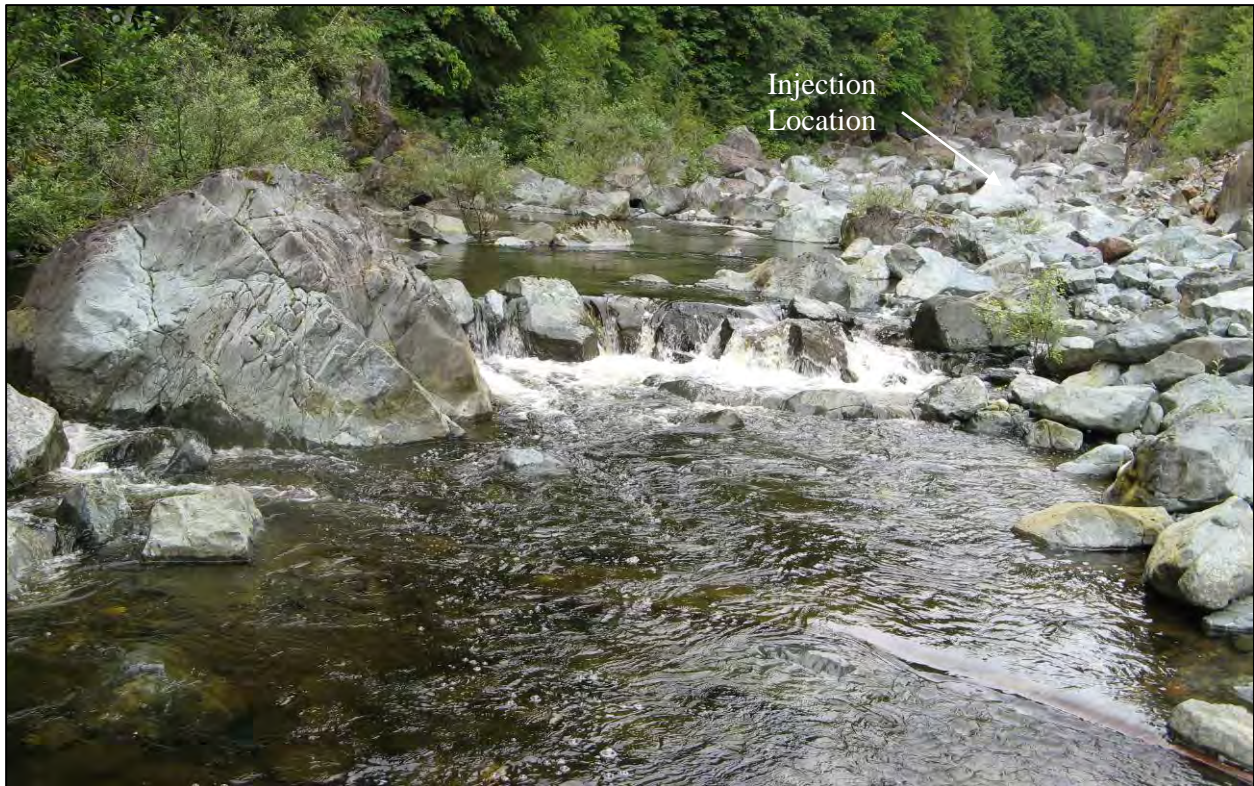
Photo 5. M1 salt dilution gauging section (looking upstream). Salt was released in the vicinity of the arrow and intercepted by the conductivity meter immediately below the photographer (distance ~ 75 m). Photo taken Aug. 26, 2008; gauged flow was 0.456 \text{ m}^3/\text{s} .
