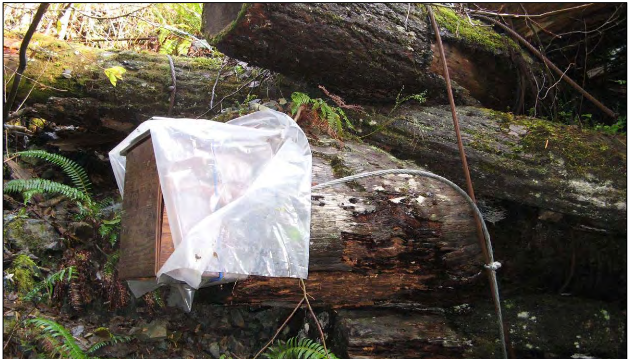
Photo 4. Plywood housing for the T1 logger and battery on Sinn Fein Creek. The box was nailed to the Sinn Fein bridge abutment; the transducer cable was sheathed in wire rope which was shackled to the bridge cables. The transducer was bolted to a heavy metal anchor situated in a pool under the bridge.
