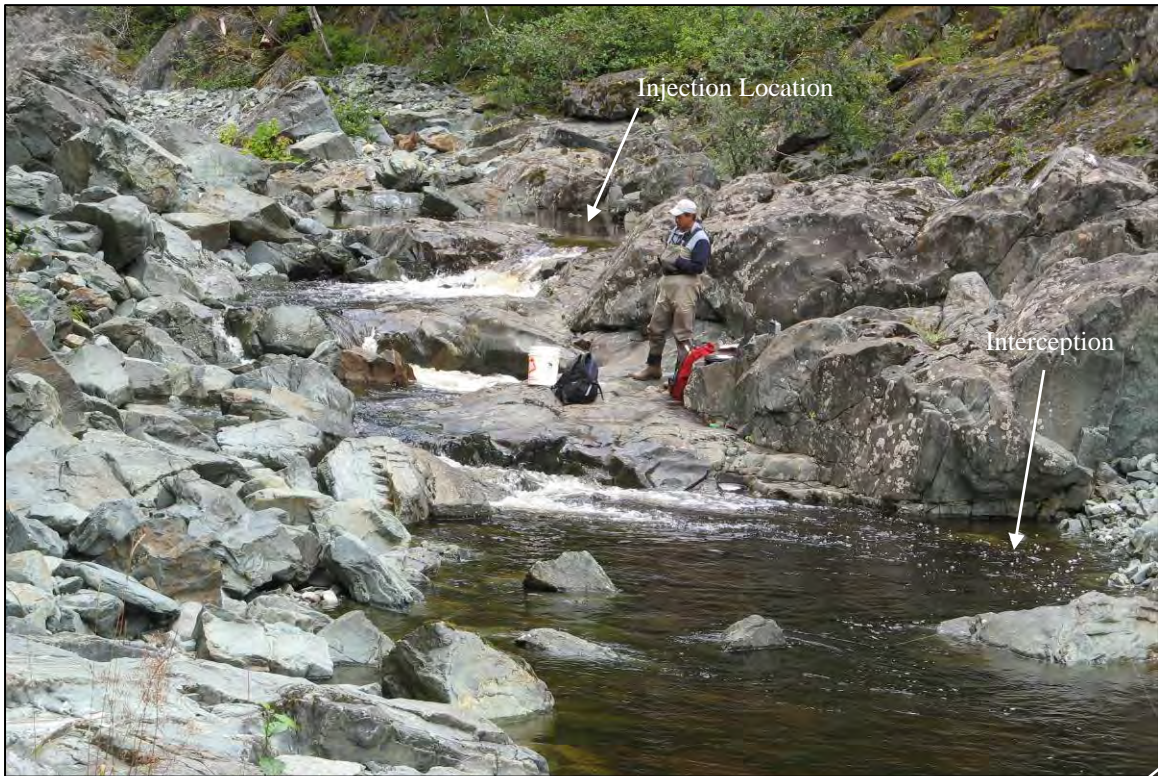
Photo 7. M3 salt dilution gauging section (looking upstream). Salt is released at the top of the cascade and intercepted by the conductivity meter at the arrow. Photo taken Aug. 26, 2008; gauged flow 0.246 m 3 /s.
