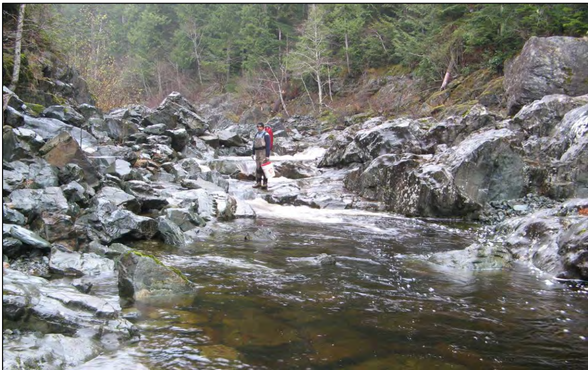
Photo 6. M3 salt dilution gauging section (looking upstream). Photo taken Nov. 27, 2008; gauged flow 0.404 m 3 /s.
