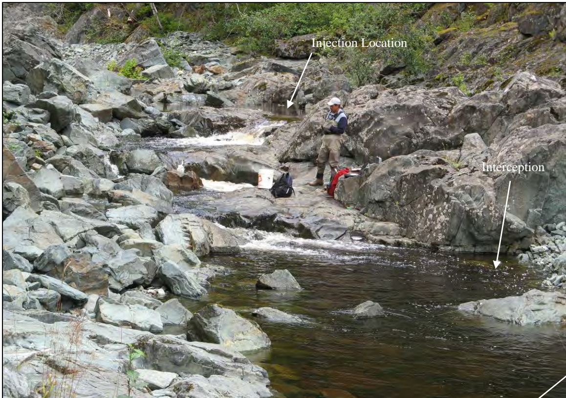
Photo 5. M3 salt dilution gauging section (looking upstream). Salt is released at the top of the cascade and intercepted by the conductivity meter at the arrow. Photo taken Aug. 26, 2008; gauged flow 0.246 m 3 /s.
