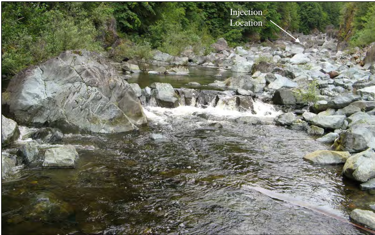
Photo 1. M1 salt dilution gauging section (looking upstream). Salt is released in the vicinity of the arrow and intercepted by the conductivity meter immediately below the photographer (distance ~ 75 m). Photo taken Aug. 26, 2008; gauged flow 0.456 \text{ m}^3/\text{s} .
