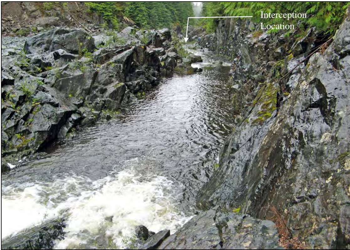
Photo 3. M2 salt dilution gauging section (looking downstream). Salt is released in the cascade and intercepted by the conductivity meter at the arrow. Photo taken Aug. 27, 2008; gauged flow 0.925 \text{ m}^3/\text{s} .
