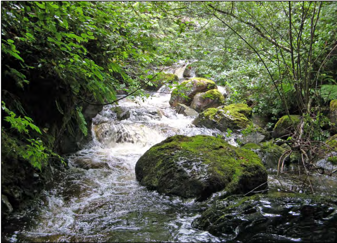
Photo 7. T1 (Sinn Fein) salt dilution gauging section (looking upstream). Salt is released 40 m upstream (beyond the trees) and intercepted by the conductivity meter at the foot of the photographer. Photo taken Aug. 27, 2008; gauged flow 0.348 m 3 /s.
