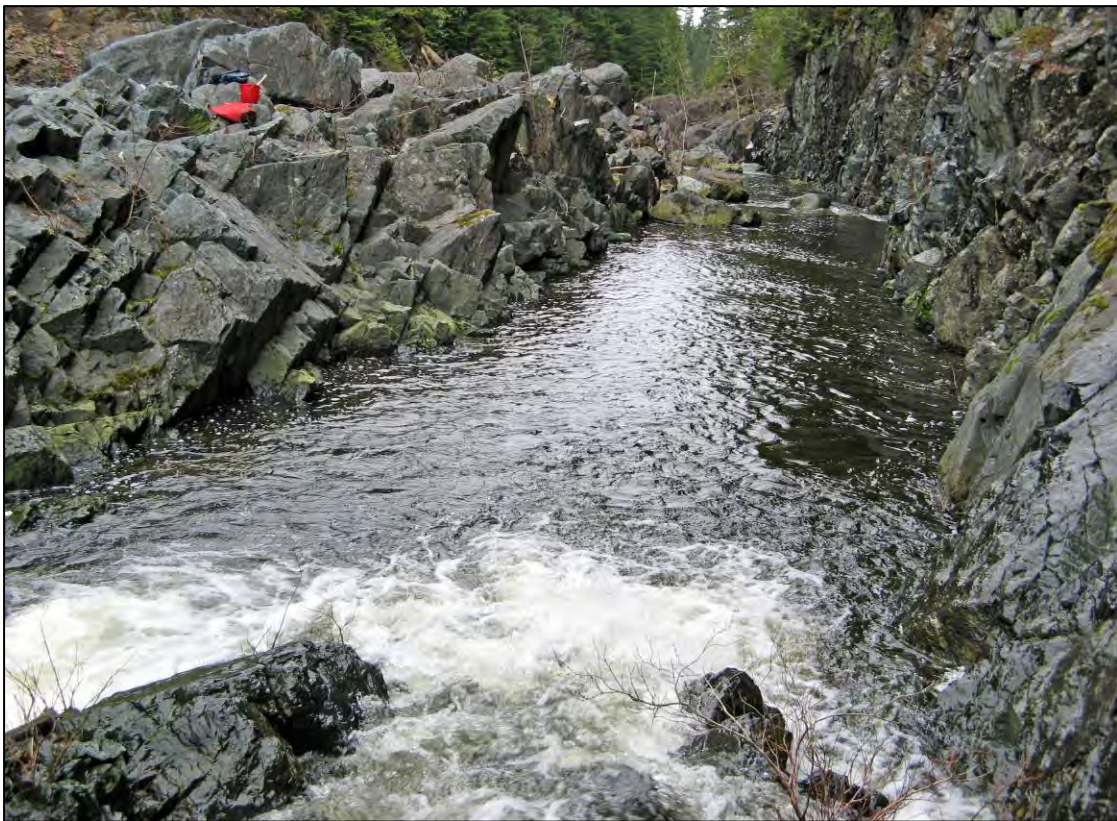
Photo 4. M2 salt dilution gauging section (looking downstream). Photo taken Nov. 27, 2008; gauged flow 0.682 \text{ m}^3/\text{s} .
