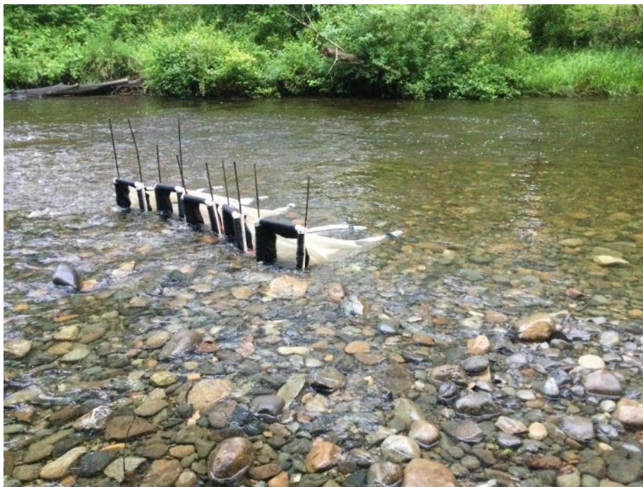
Figure 4. View of invertebrate sampling drift nets across the stream from river right towards QUN-IV, July 06, 2022.
