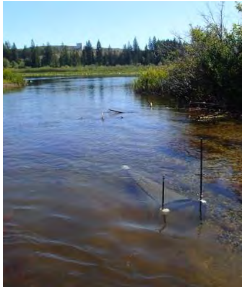
Figure 5. Drift net secured in the Quinsam River to sample benthic macroinvertebrates upstream of Middle Quinsam Lake (background).
