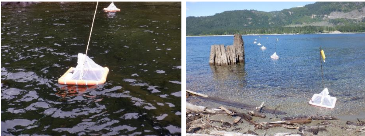
Figure 6. Left: floating trap deployed at Lower Campbell Reservoir (LCR-EIV03) on May 26, 2021; right: floating traps deployed at varying distances from shoreline, and inside and outside the drawdown zone at Upper Campbell Reservoir (UCR-EIV02) on May 20, 2021.
