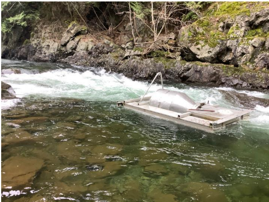
Figure 2. Rotary Screw Trap (RST) during operation in 2022 at base of Elk Canyon at 10 m 3 /s (Position #2).
