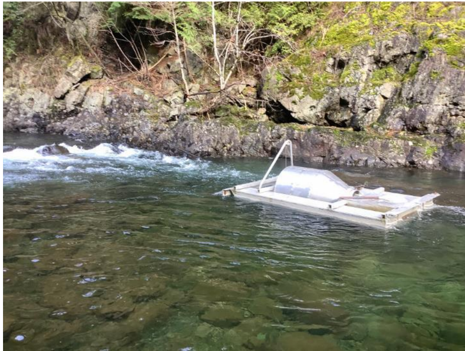
Figure 1. Rotary Screw Trap (RST) during operation in 2022 at base of Elk Canyon at 4 m 3 /s (Position #1).
