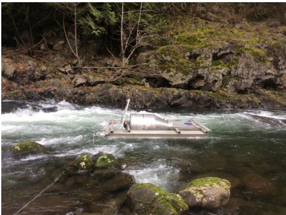
Figure 2. Rotary Screw Trap (RST) during operation in 2021 at base of Elk Canyon at 10 m 3 /s (Position #2).
