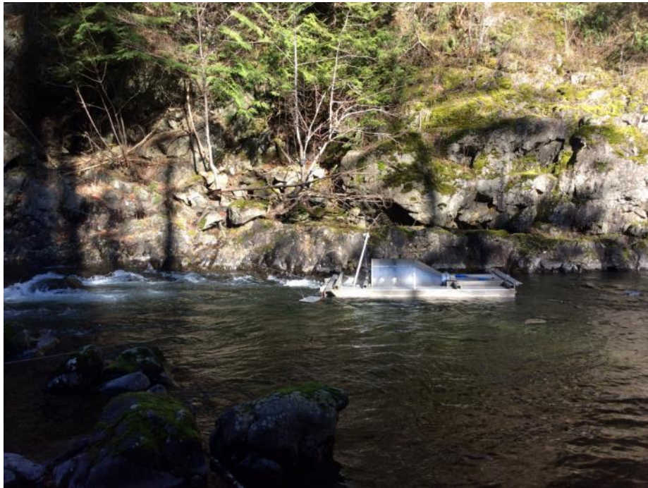
Figure 1. Rotary Screw Trap (RST) during operation in 2021 at base of Elk Canyon at 4 m 3 /s (Position #1).
