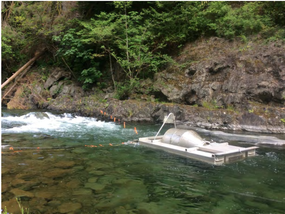
Figure 5. Rotary Screw Trap (RST) during operation at base of Elk Canyon at 4 \text{ m}^3/\text{s} low water conditions (Position #3).
