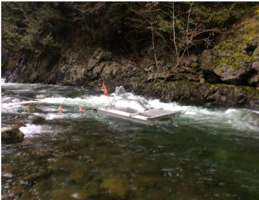
Figure 3. Rotary Screw Trap (RST) during operation at base of Elk Canyon at 10 m 3 /s (Position #2).
