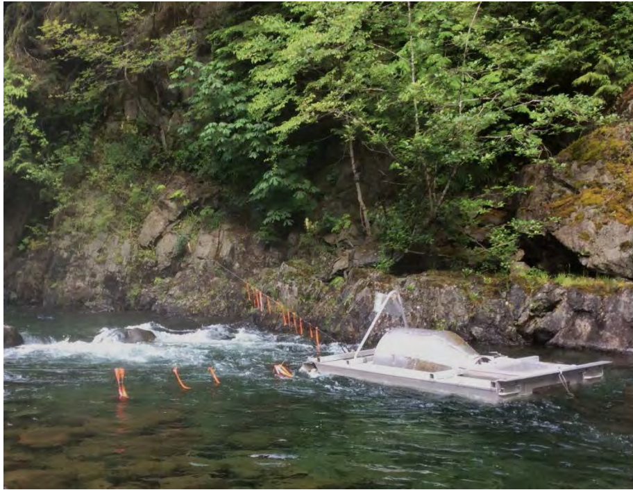
Figure 2. Rotary Screw Trap (RST) during operation at base of Elk Canyon at 4 m 3 /s (Position #1).
