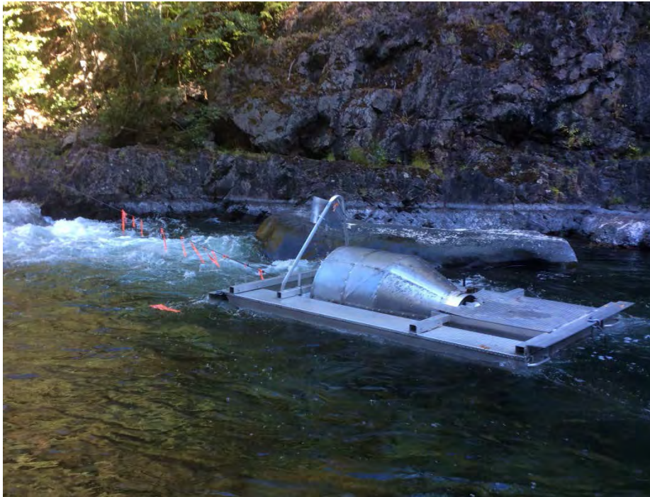
Figure 4. Rotary Screw Trap (RST) during operation at base of Elk Canyon at 4 m 3 /s low water conditions (Position #3).
