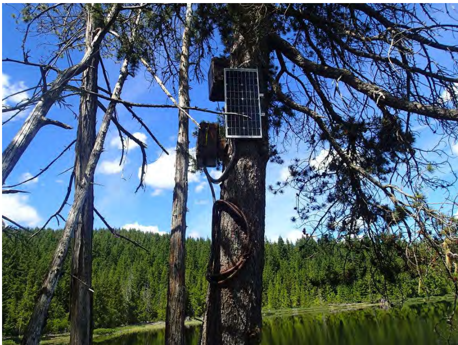
Figure 2. Brewster Lake Gauging Station (BRE-LG01): Data logger, solar panel, and battery box tree mounted, as installed on June 30, 2014.
