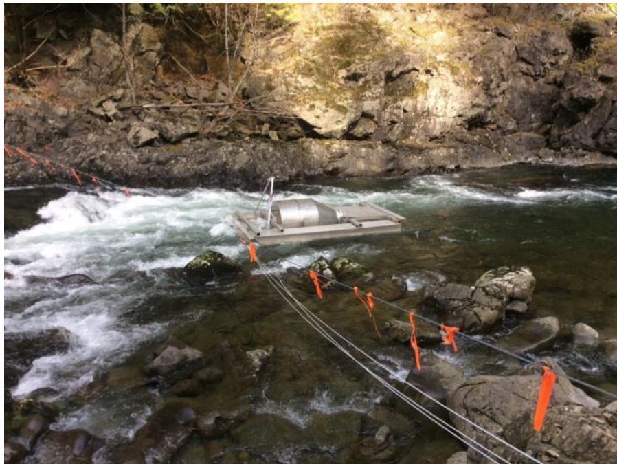
Figure 3. Rotary Screw Trap (RST) during operation at base of Elk Canyon at 7 m 3 /s (Position #2).
