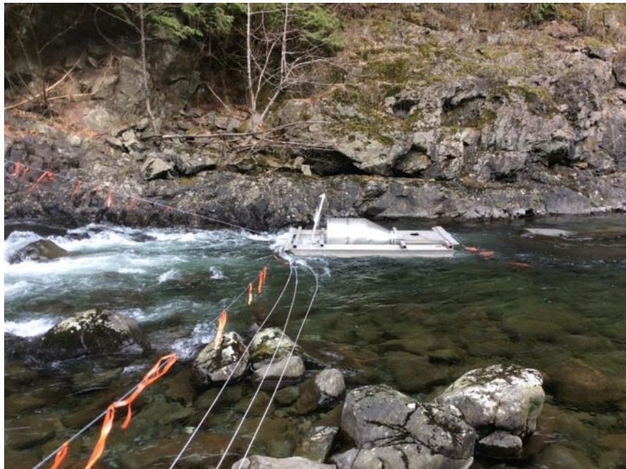
Figure 2. Rotary Screw Trap (RST) during operation at base of Elk Canyon at 4 m 3 /s (Position #1).
