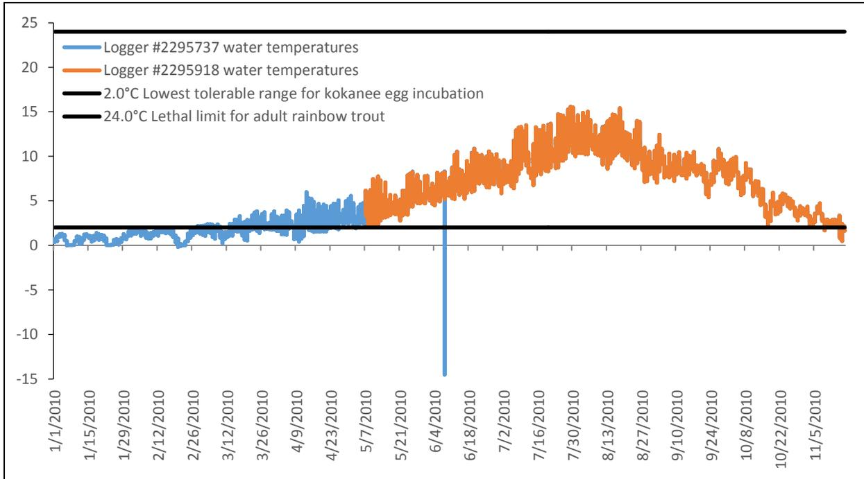
**Figure 23.** Water temperatures recorded from January to November 2010 at Site 4 (control) from logger #2295737, and logger #2295918.
