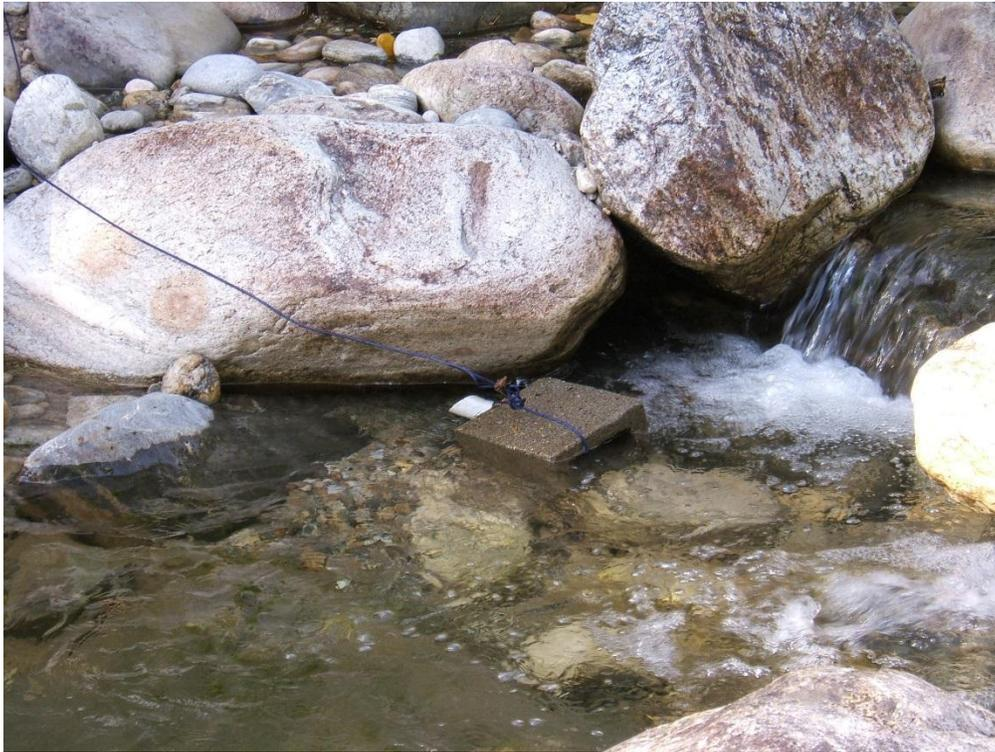
**Photo 1:** Example of a temperature logger secured within a PVC pipe and anchored inside a cinder block. Photo taken September 21, 2009
