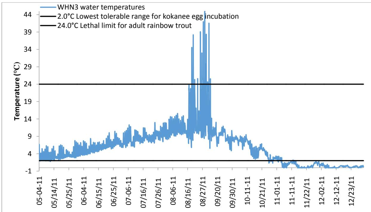
**Figure 18.** Water temperatures recorded from May to December 2011 at Site 3 from the WHN3 temperature logger. Data measured at 60 minute intervals.
