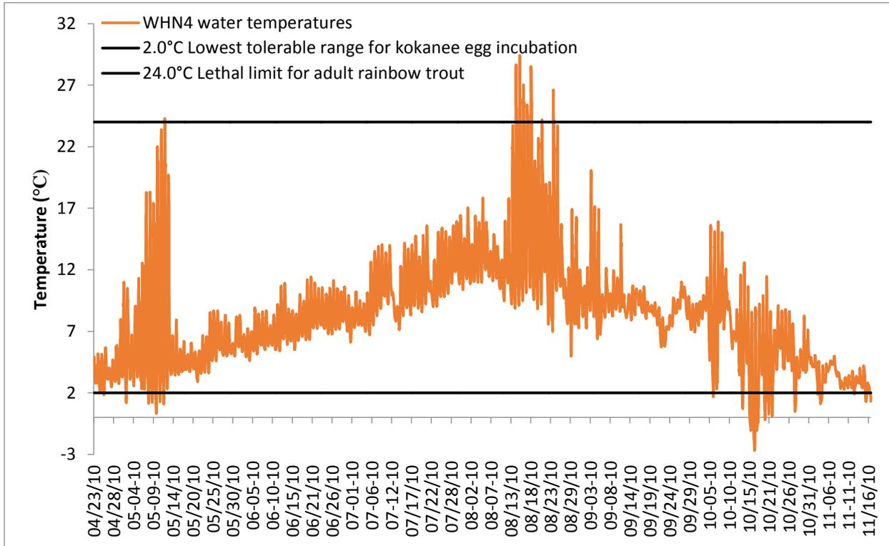
**Figure 17.** Water temperatures recorded from April to November 2010 at Site 3 from the WHN4 temperature logger. Data measured at 30 minute intervals.
