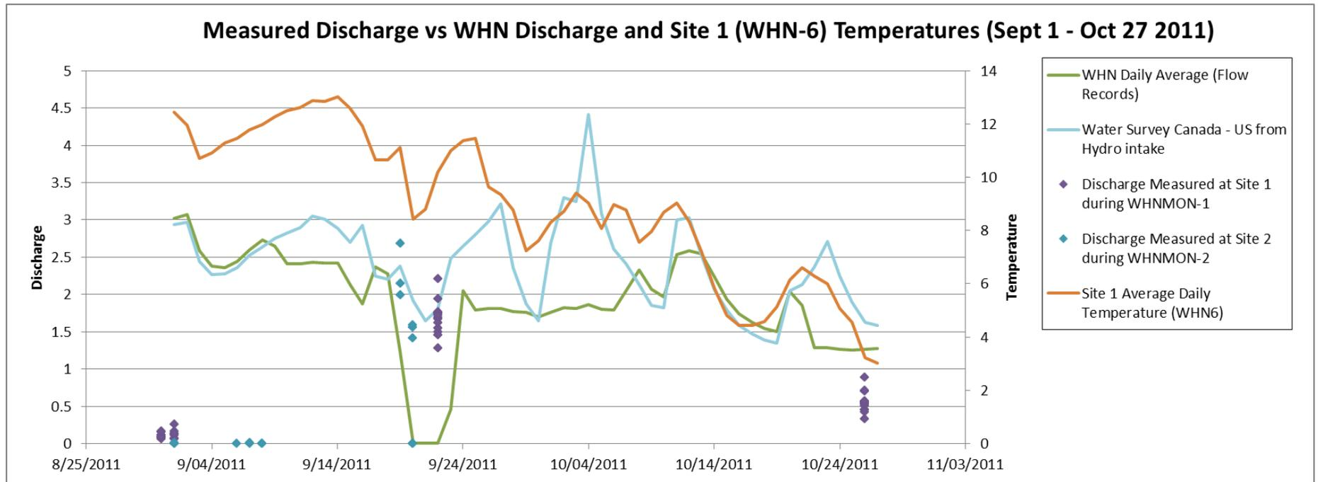
Figure 2. Measured discharge vs. WHN discharge and Site 1 (WHN6) temperatures September 1 to October 27, 2011
