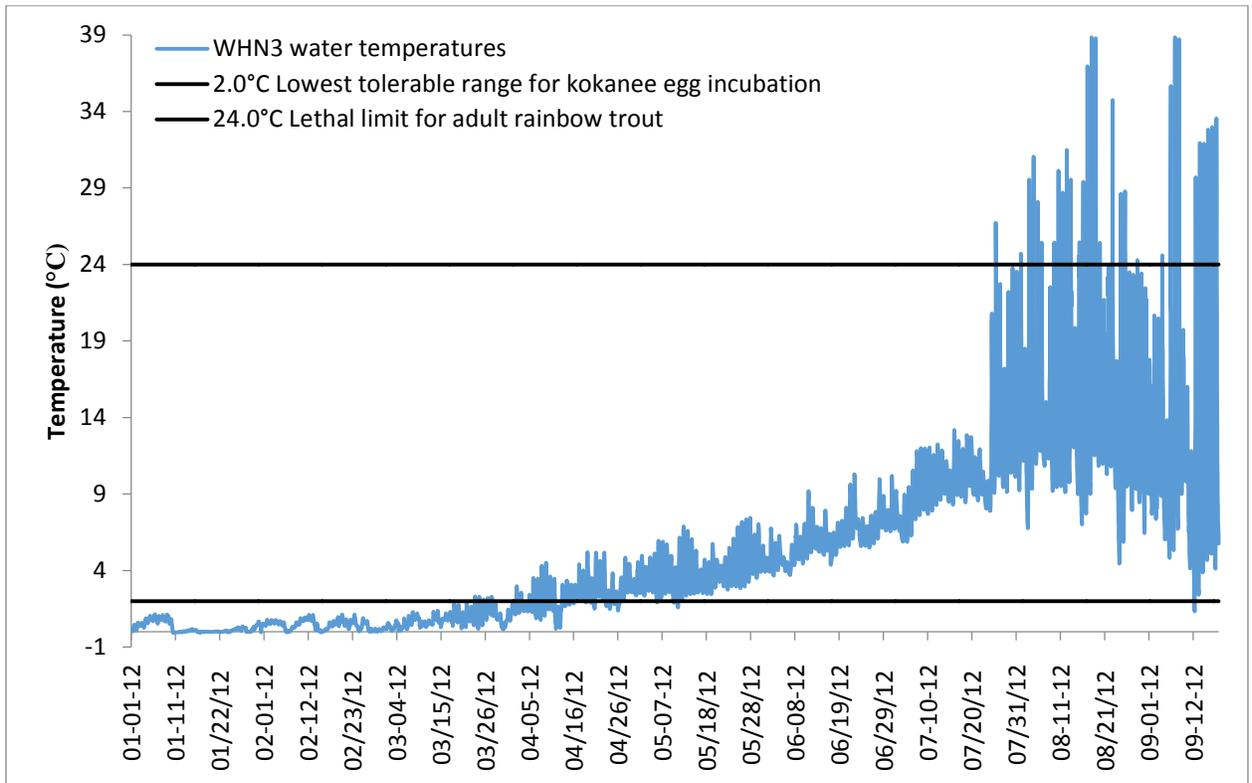
**Figure 20.** Water temperatures recorded from January to September 2012 at Site 3 from the WHN3 temperature logger. Data measured at 60 minute intervals.
