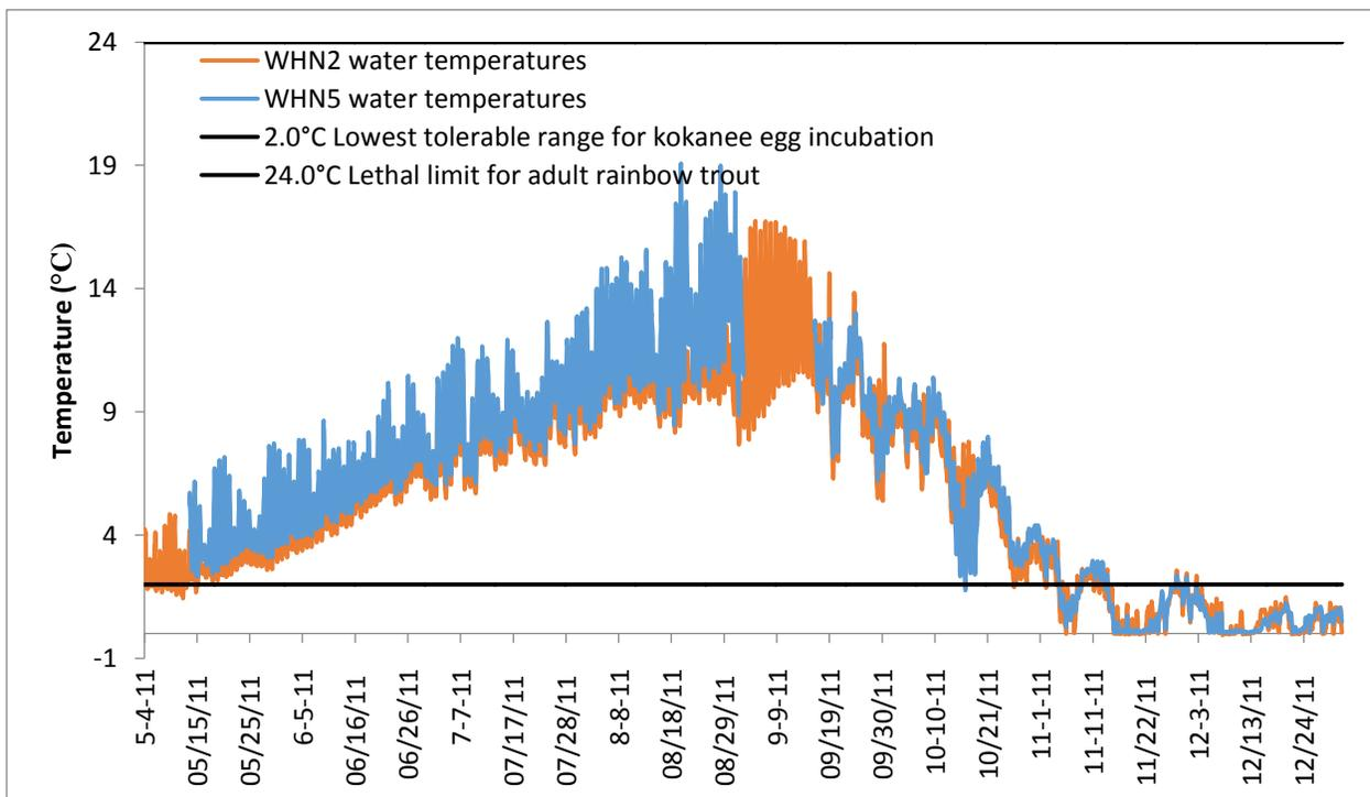
**Figure 12.** Water temperatures recorded from May to December 2011 at Site 2 from the WHN2 temperature logger, and May to August, and September to December 2011 from the WHN5 temperature logger.
