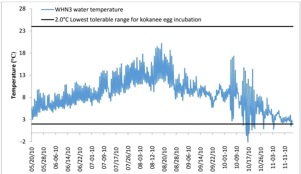
**Figure 16.** Water temperatures recorded from May to November 2010 at Site 3 from the WHN3 temperature logger. Data measured at 60 minute intervals.
