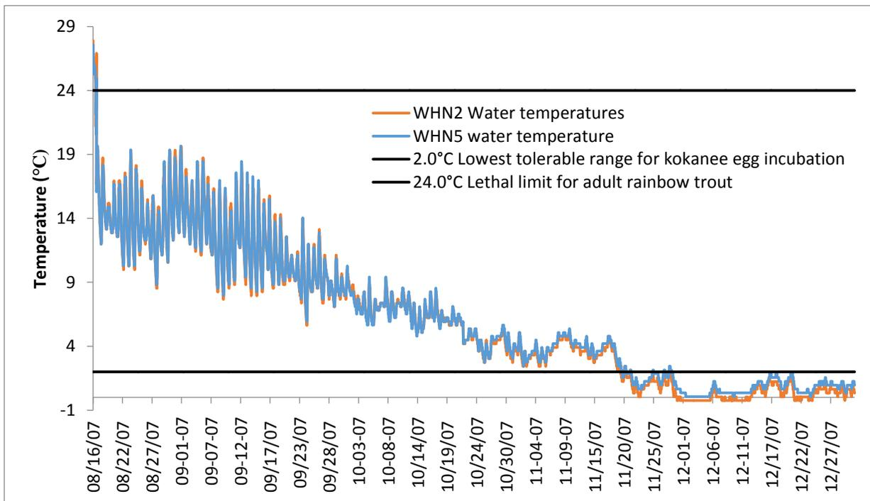
**Figure 8.** Water temperatures recorded from August to December 2007 at Site 2 from both WHN2 and WHN5 temperature loggers.
