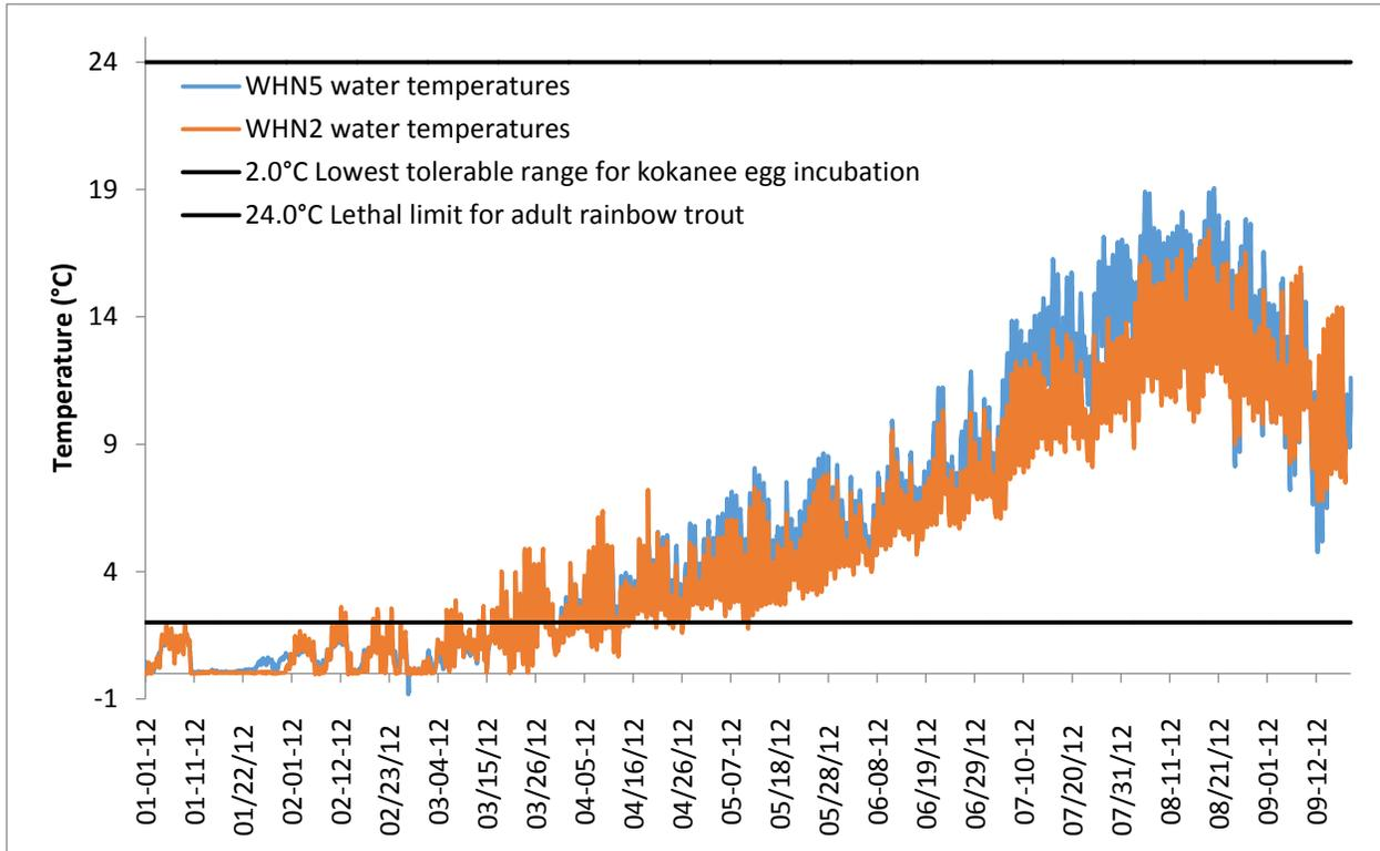
**Figure 13.** Water temperatures recorded from January to September 2012 at Site 2 from both WHN2 and WHN5 temperature loggers.
