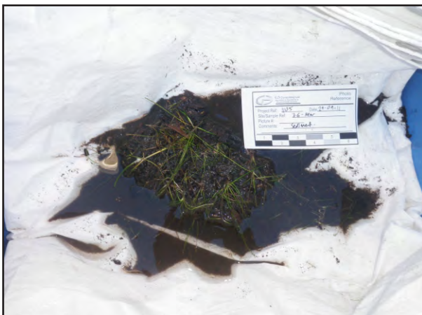
Photo 3-5: Sediment sample taken from Site 3-6 centre nearshore (September 29, 2011)
