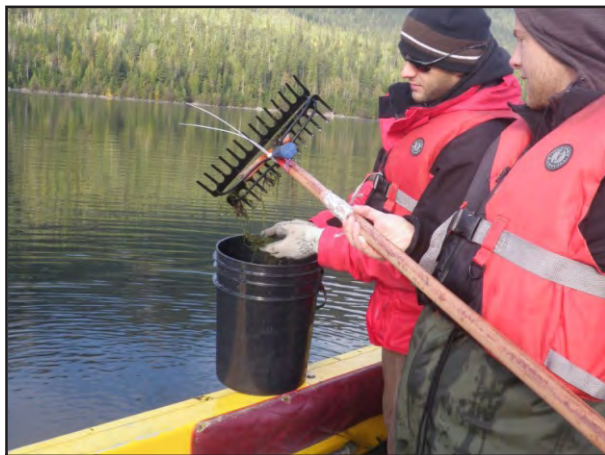
Photo 2-7: Collecting submerged macrophytes using a macrophyte sampling rake
