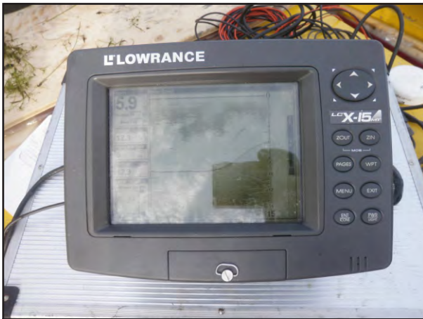
Photo 2-3: Digital Lowrance LCX-15MT depth sounder interfacing directly to an omnistar DGPS receiver used to view and record bathymetry data
