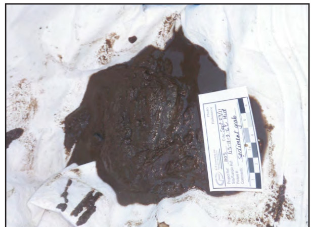
Photo 3-6: Sediment sample taken from Site 3-6 centre mid distance from shore (September 29, 2011)
