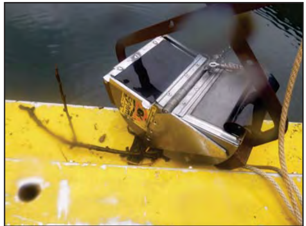
Photo 2-4: Petit ponar used to collect sediment samples
