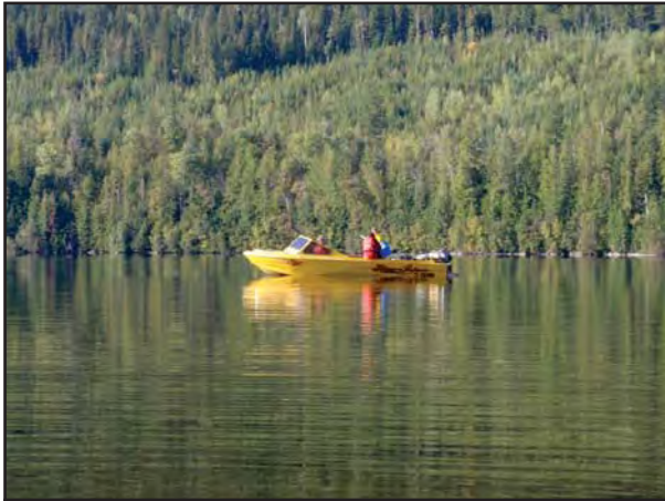
Photo 2-1: Looking at the 6.7 m aluminum field vessel powered by a 340 HP inboard jet drive engine
