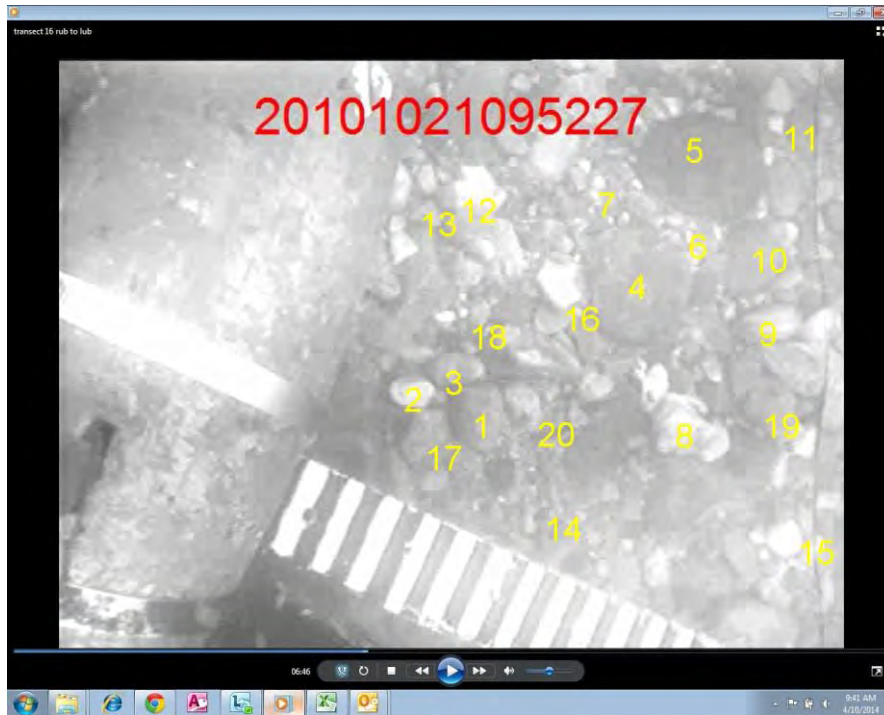
Plate 7: Screen capture from the underwater videography survey showing the substrate particles selected for measurement.
