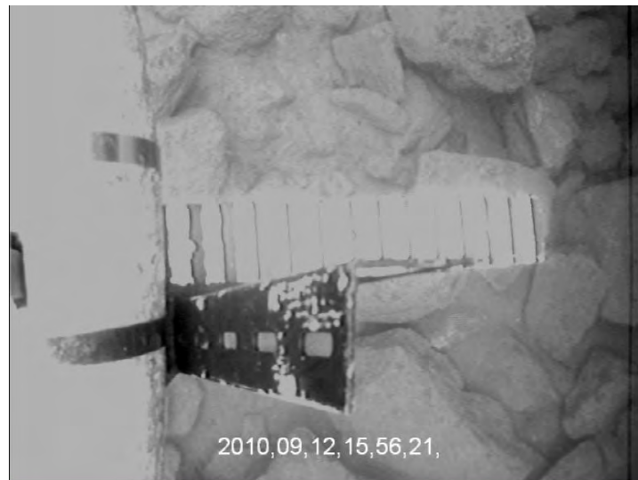
Figure 4: A typical video frame capture at transect 21. The object on the left is the lead fish and the bright object in the center of the frame is the scaling bar.
