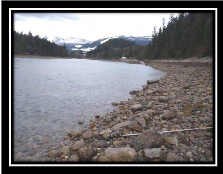
Photo 1: Bottom of Station 1 standpipe housing (Reach 4) unable to capture the lowest water levels due to the absence of appropriate shoreline with vertical rock faces or steep banks. Photo taken April 27, 2011.
