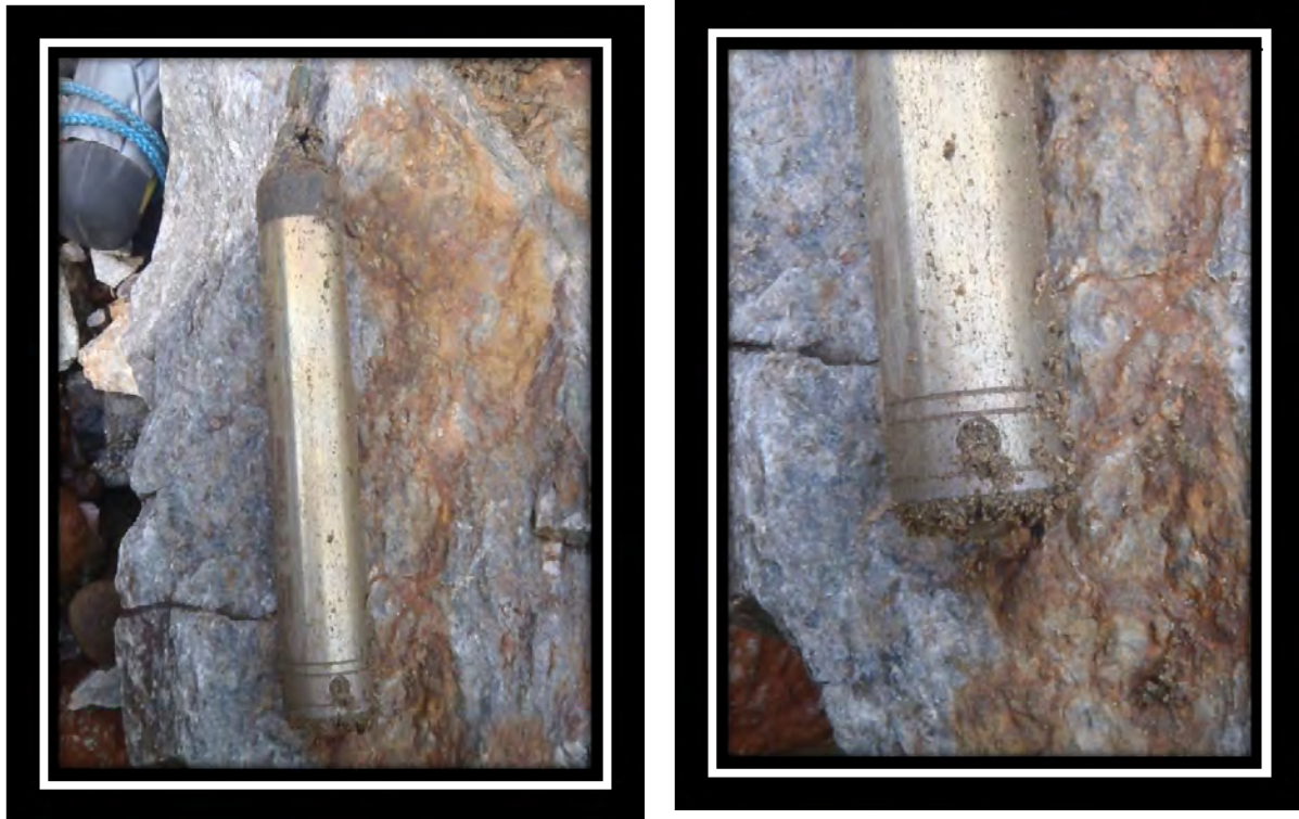
Photos 5 & 6: Station 1 data logger showing a considerable amount of sediment on the data logger housing and the sensor affecting data readings. Photo taken April 27, 2011.
