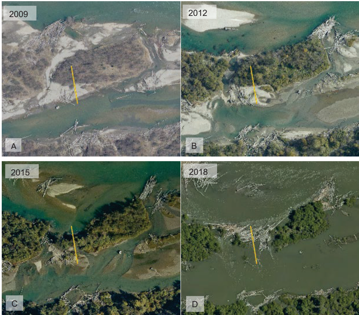
Figure 3-15: D3T20 transect area showing the mid-channel bar and the active channel in March 2009 (A), same place in October 2012 (B), partial scour by September 2015 (C) and completely scoured by June 2018 (D). The mid-channel bar where the transect line was set up in 2009 was gone in 2017 but the next air photo scheduled flight was in 2018.
