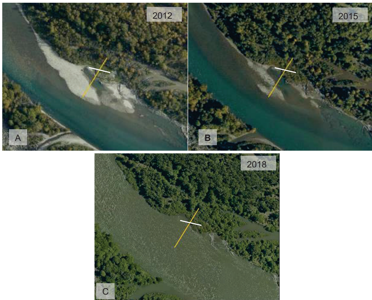
Figure 3-16: D5T16 transect area showing the partial mid-channel bar and the active channel in October 2012 (A), a small amount of scour of main bank next to the small backchannel by September 2015 (B) and complete scour of the partial mid-channel bar and a small area of the Pre-Alt S73 recruitment zone in June 2018 (C). The white line indicates the river's edge in 2018 for the bisection of the transect.
