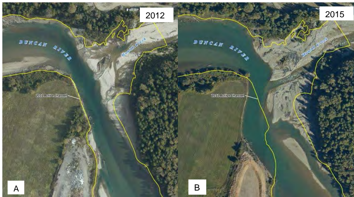
Figure 3-24: Air photos of Duncan Segment 4, Hamill Creek area in October 2012 (A) and the same area in September 2015 (B). The active channel delineation is for 2012.
