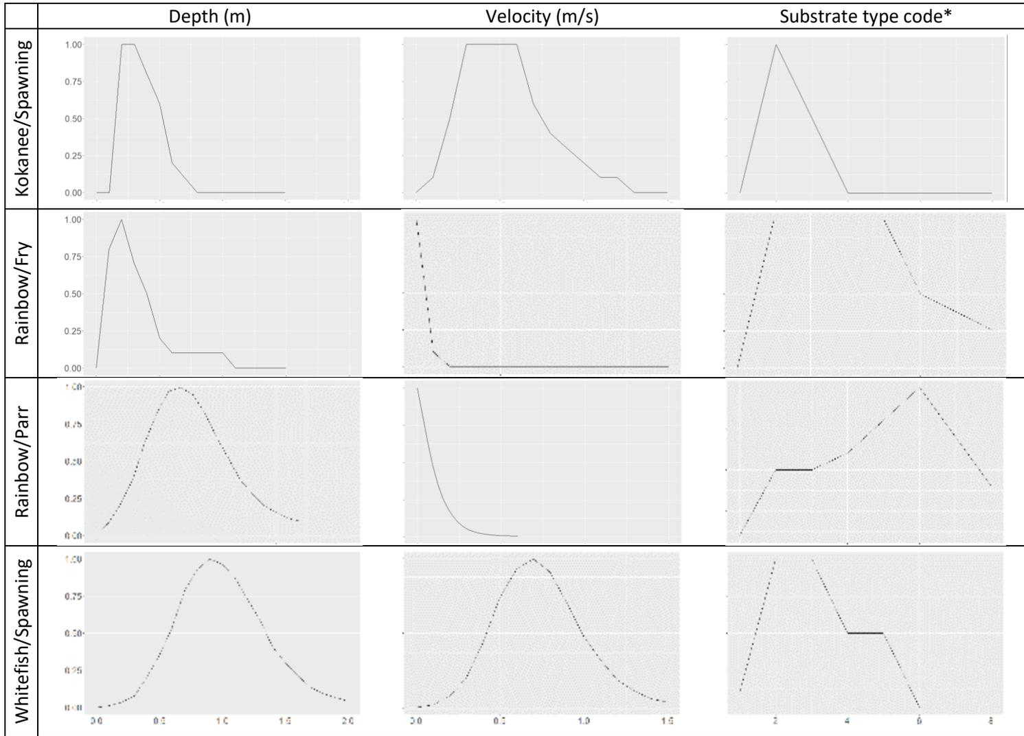
Figure 4-2: Habitat Use Curves (HUC) used in model T2D\_2020 to compute Habitat Suitability Index (HSI) and Weighted Usable Area for each species/life stage. Data from the corresponding project (DDMMON-2 for RT and MW, and DDMMON-4 for KO). \* See Table 4-2 for details on substrate type codes.
