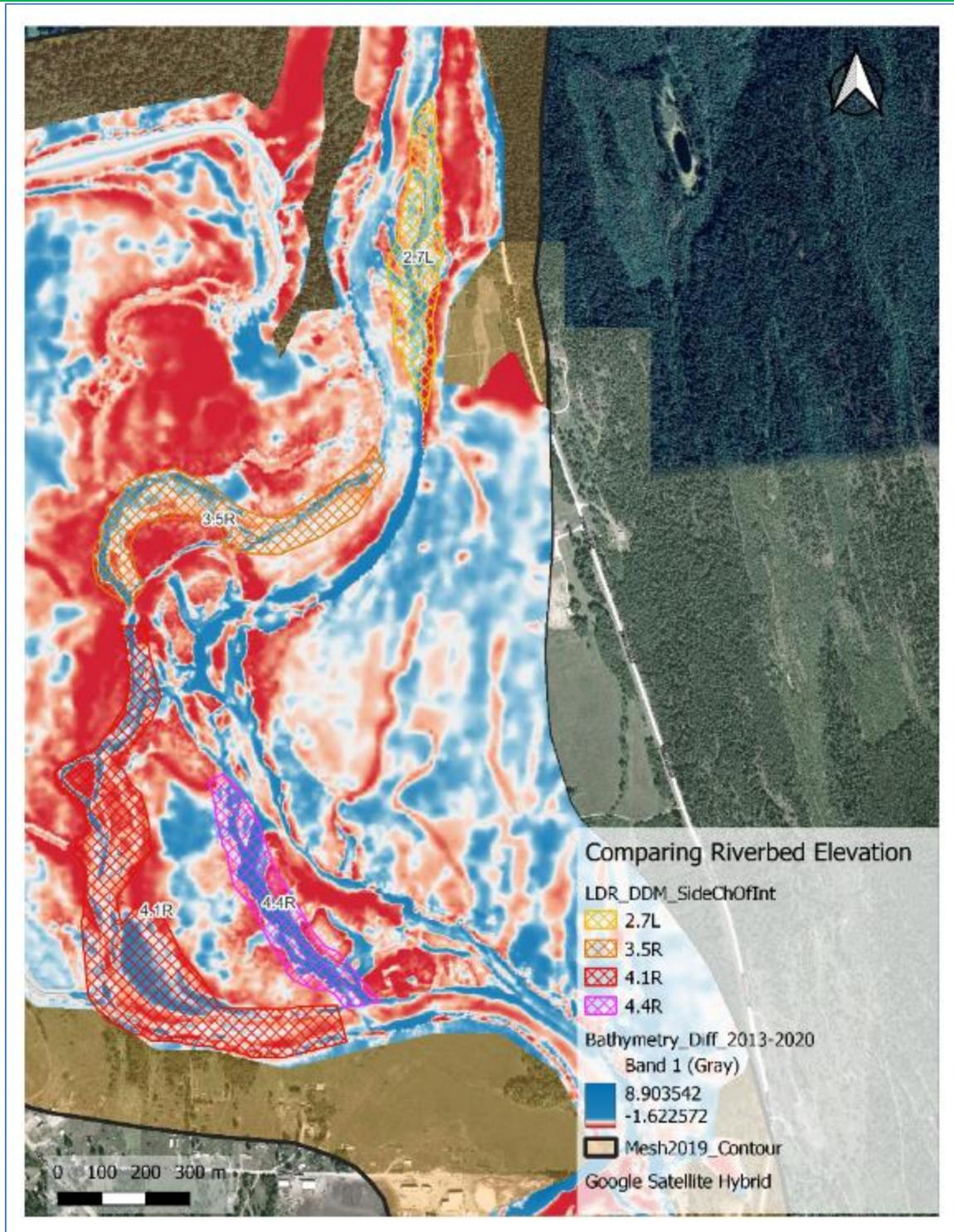
Figure A - 4: Detail of bathymetric differences (m) between 2013 and 2020 riverbeds. Blue indicates a positive difference, meaning the elevation at that coordinate was higher in 2013. Red indicates the coordinate's elevation was higher in 2020. Most of the river mainstem is blue, meaning the 2020 bathymetric data represents, in general, a deeper mainstem in this section.
