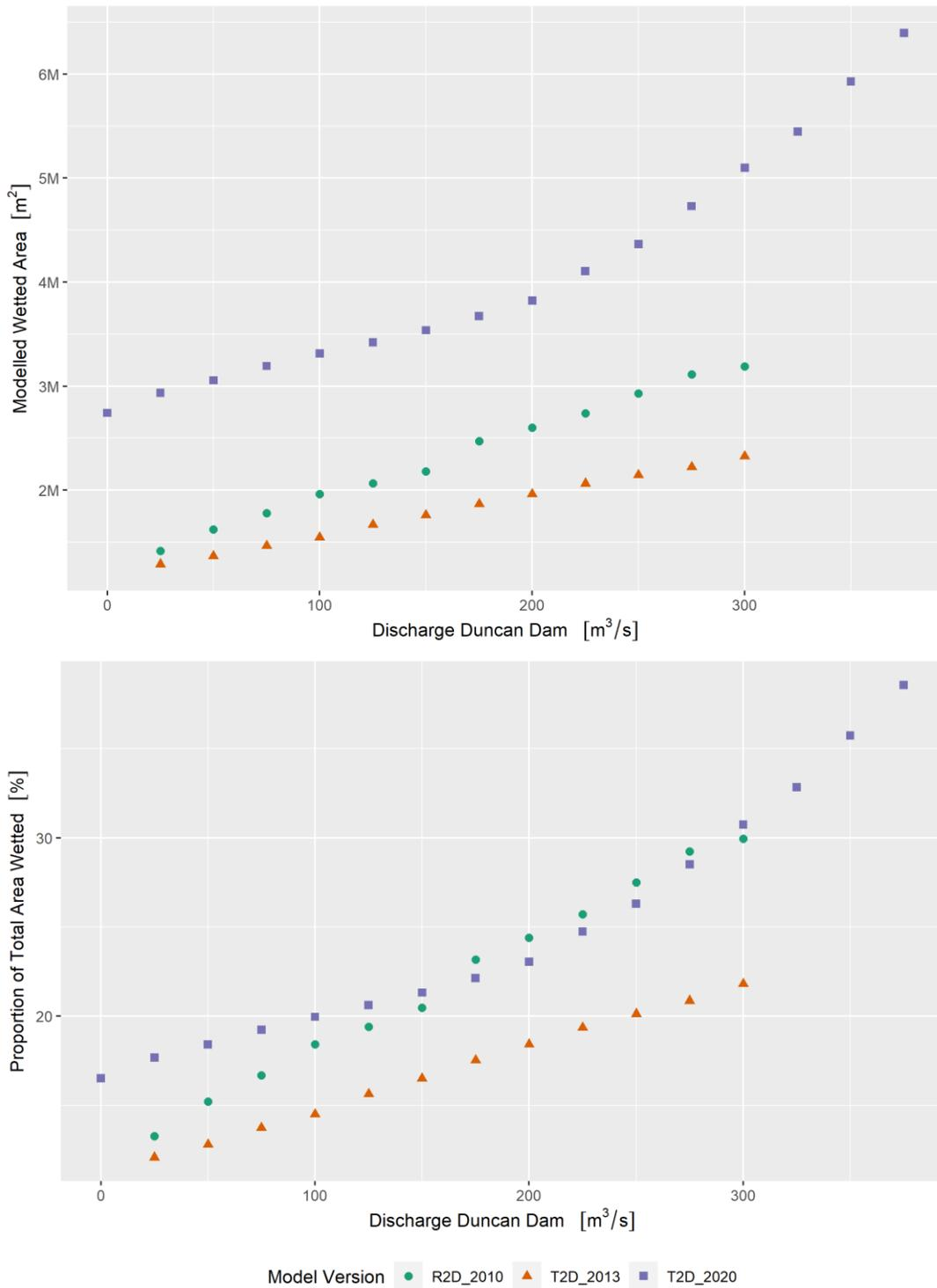
**Figure 4-1: Simulated Wetted Area: nominal (top) and relative to the extent of modelled area (bottom); predicted by the corresponding model version, for a 20 m³/s discharge from the Lardeau River.**
