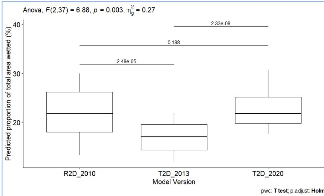
**Figure 5-5: Boxplot comparing F-Test results for the predicted proportion of wetted area by model. T2D\_2020 = 2020 Telemac 2D Update; T2D\_2013 = 2013 T2D Model; R2D\_2010 = River 2D 2010 Model.**
