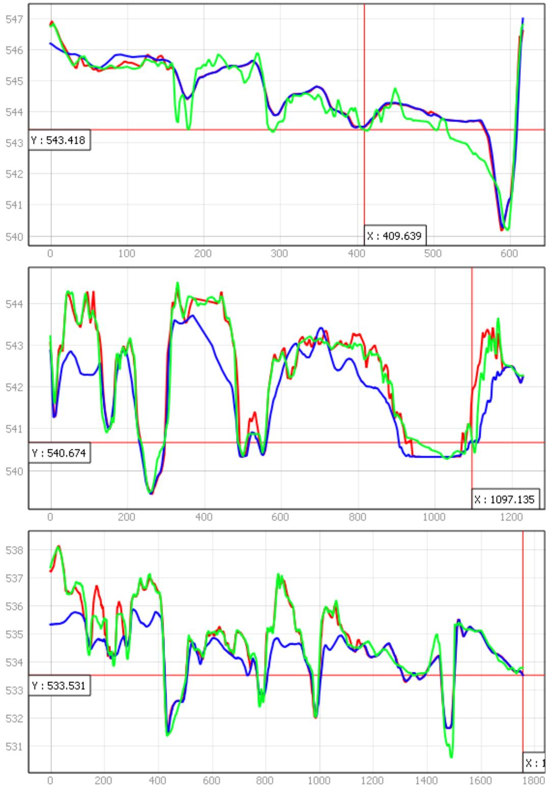
**Figure A - 3: Elevation profile comparison, in m, for bathymetric data sets. 2008 (Red), 2013 (Blue), 2020 (green). Along Side Channel 1.1R (Top), across 2.7L (Middle), and across 7.1R (Bottom). X axis represents the cross-section, in m.**
