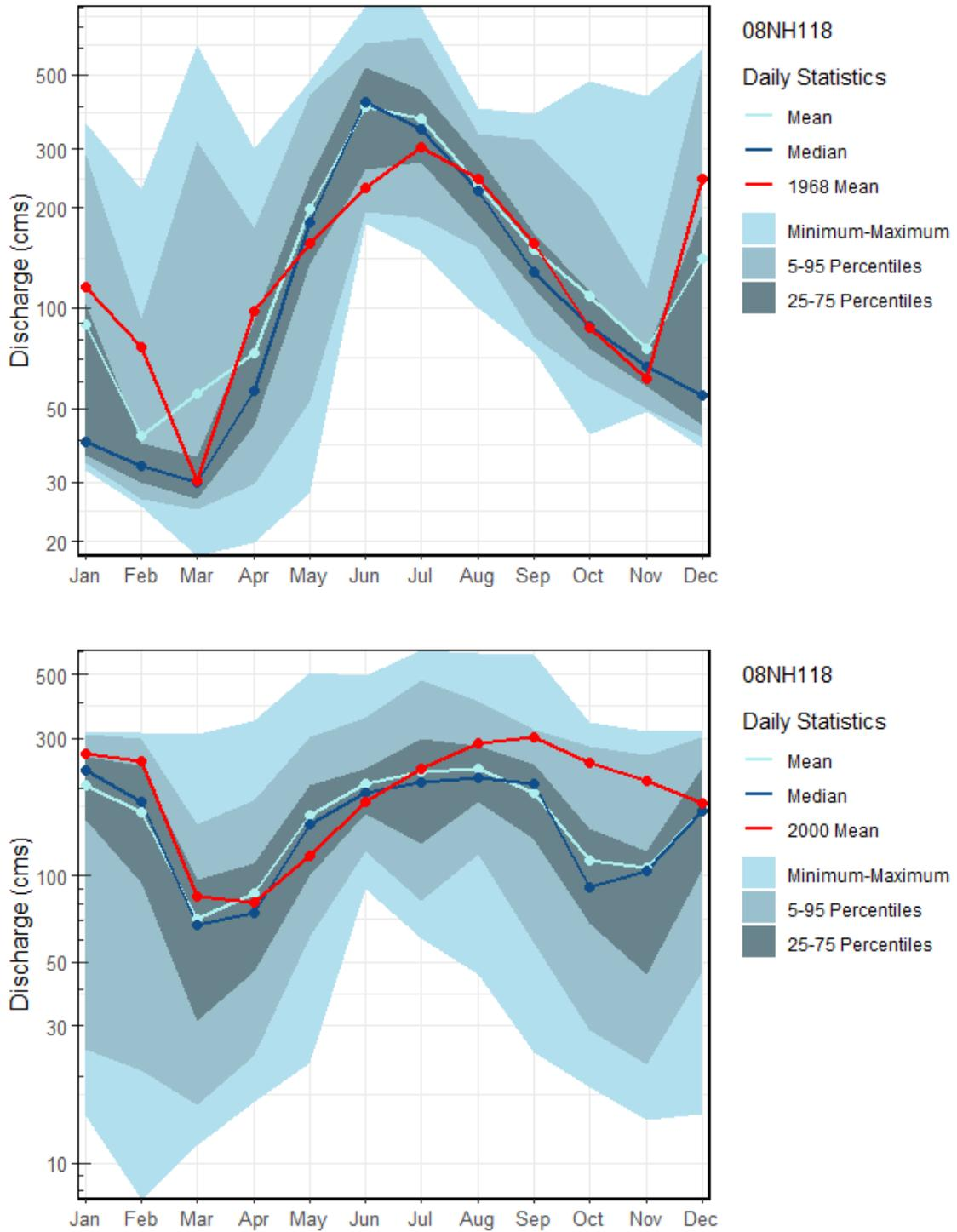
Figure 2-2: Lower Duncan River hydrograph depicting mean daily flows. Top: before, and bottom: after the construction of the Duncan Dam (1969).
