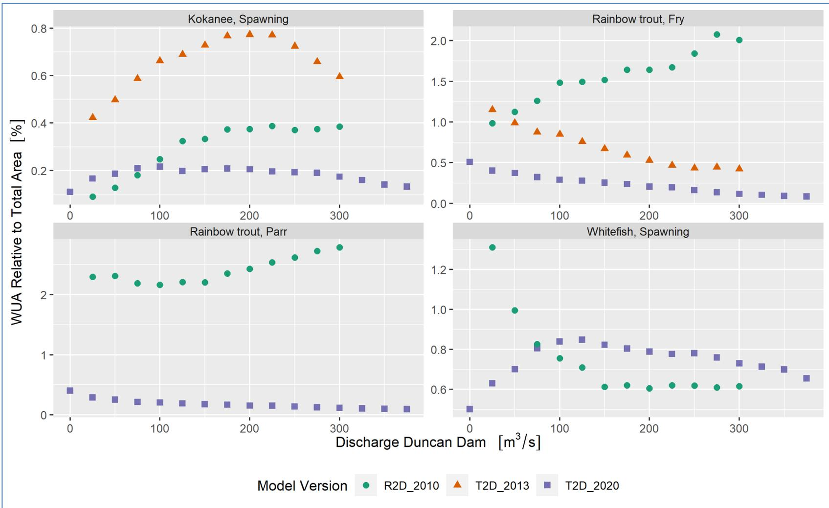
Figure 4-4: Relative WUA with respect to simulated total area for each species/life stage derived from the simulated results for depth, velocity, substrate size, and HUC. Note Y axis scale is different in each plot.
