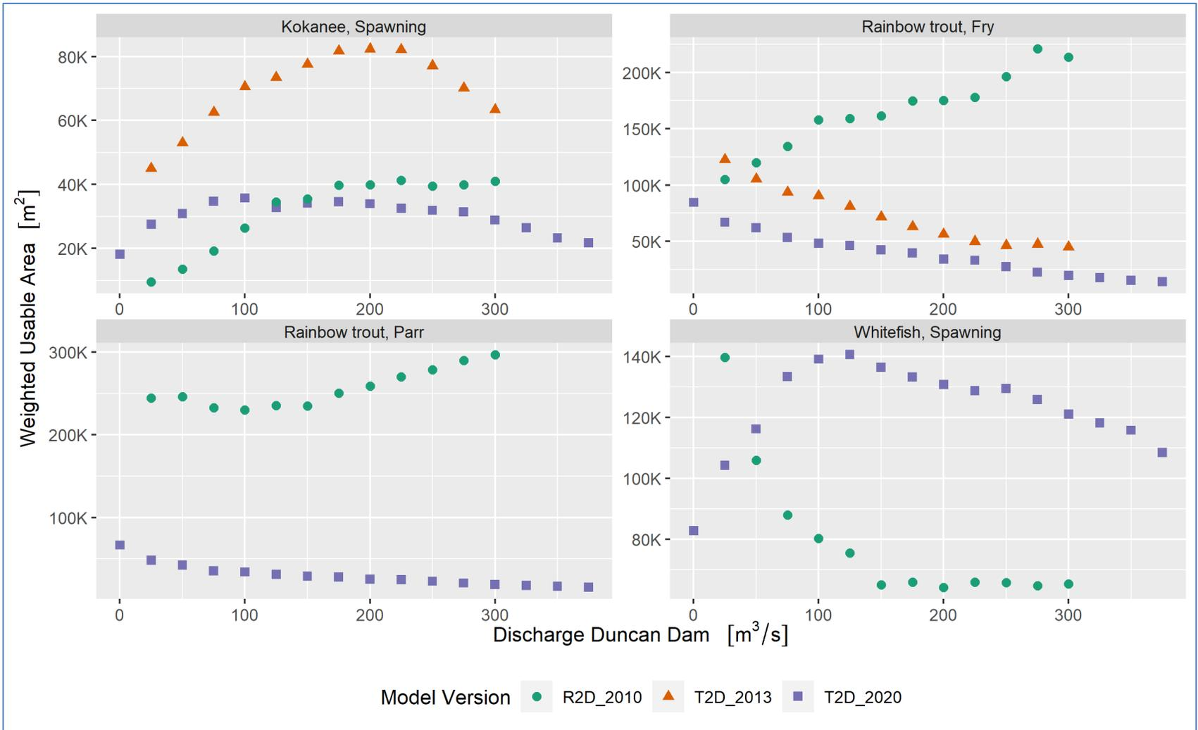
Figure 4-3: Weighted Usable Area (WUA in m²) for each species/life stage derived from the simulated results for depth and velocity, substrate size, and HUC. Note Y axis scale is different for each species/life-stage.
