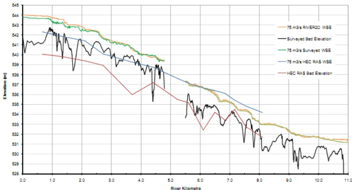
Figure 6-1: Long Profiles of the Lower Duncan River (NHC, 2010). 1D Model profiles are blue and red lines, all others relate to the 2D Model.
