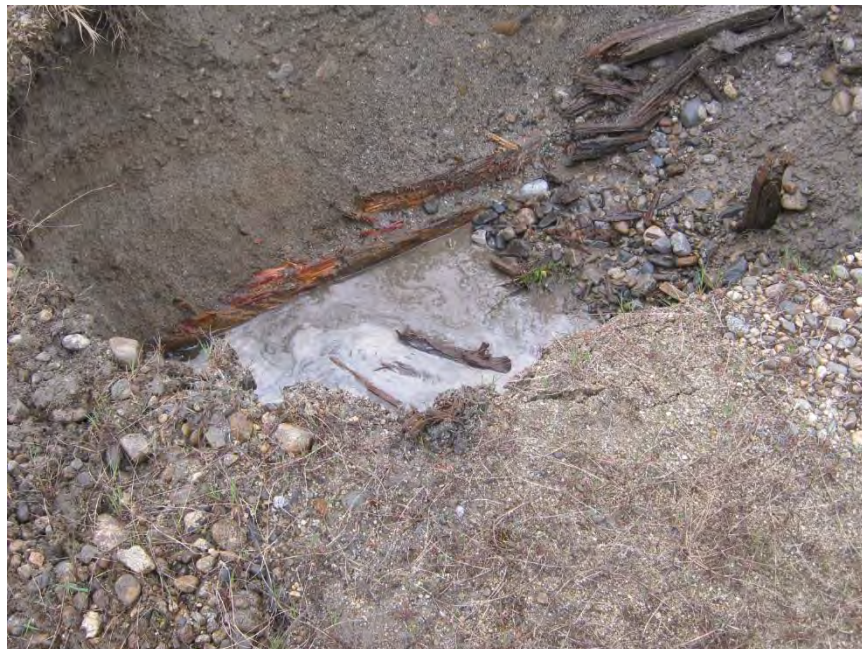
PHOTO 8: Wood debris encountered at TP17-6.
