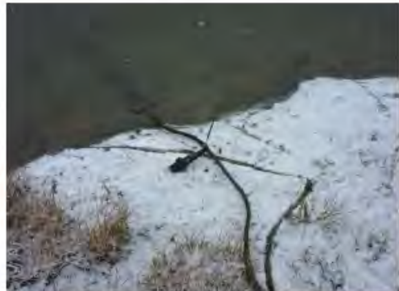
Photo 16: Anchored water level logger found downstream of Site 15a outlet.
