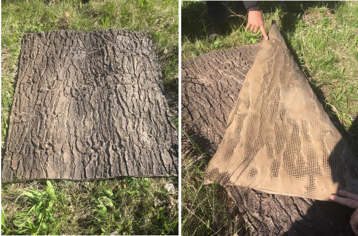
Figure 6. The exterior of a BrandenBark sheet (left) , and the interior (right), showing the mesh used to provide a grippy surface for bats to hang on to.
