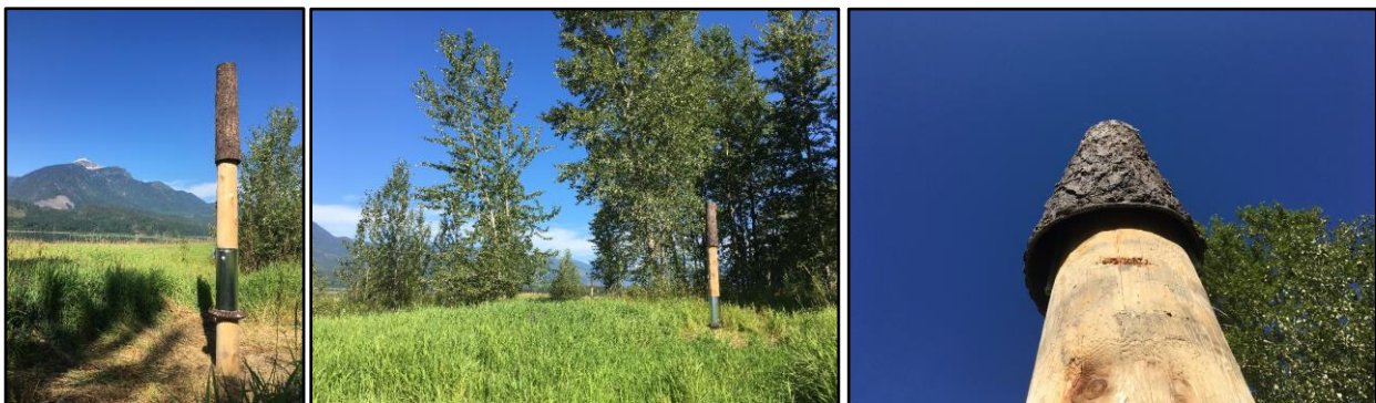
Figure 8. The two BrandenBark poles at Montana3, and looking up the cedar pole at the gap between the pole and bark.
