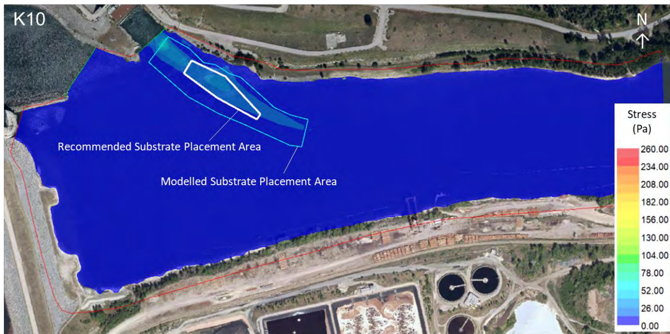
Figure 4: River2D Simulated Shear Stresses (Pa) for the K10 (Average Spawning Flow) Scenario (Extracted from Hydrodynamic Modelling by Ecofish (2020))
