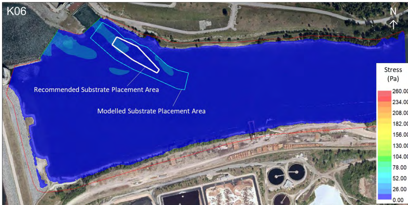
Figure 1: River2D Simulated Shear Stresses (Pa) for the K06 (Extreme high flow event: 2012) Scenario (Extracted from Hydrodynamic Modelling by Ecofish (2020))
