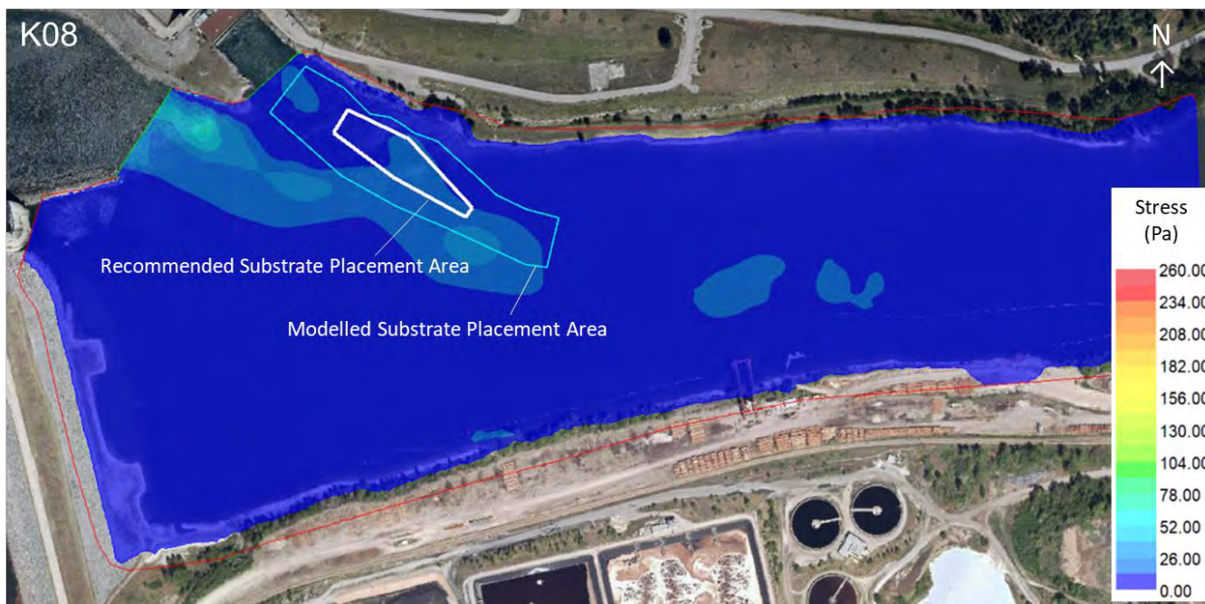
Figure 2: River2D Simulated Shear Stresses (Pa) for the K08 (Extreme high flow event: 1997) Scenario (Extracted From Hydrodynamic Modelling by Ecofish (2020))
