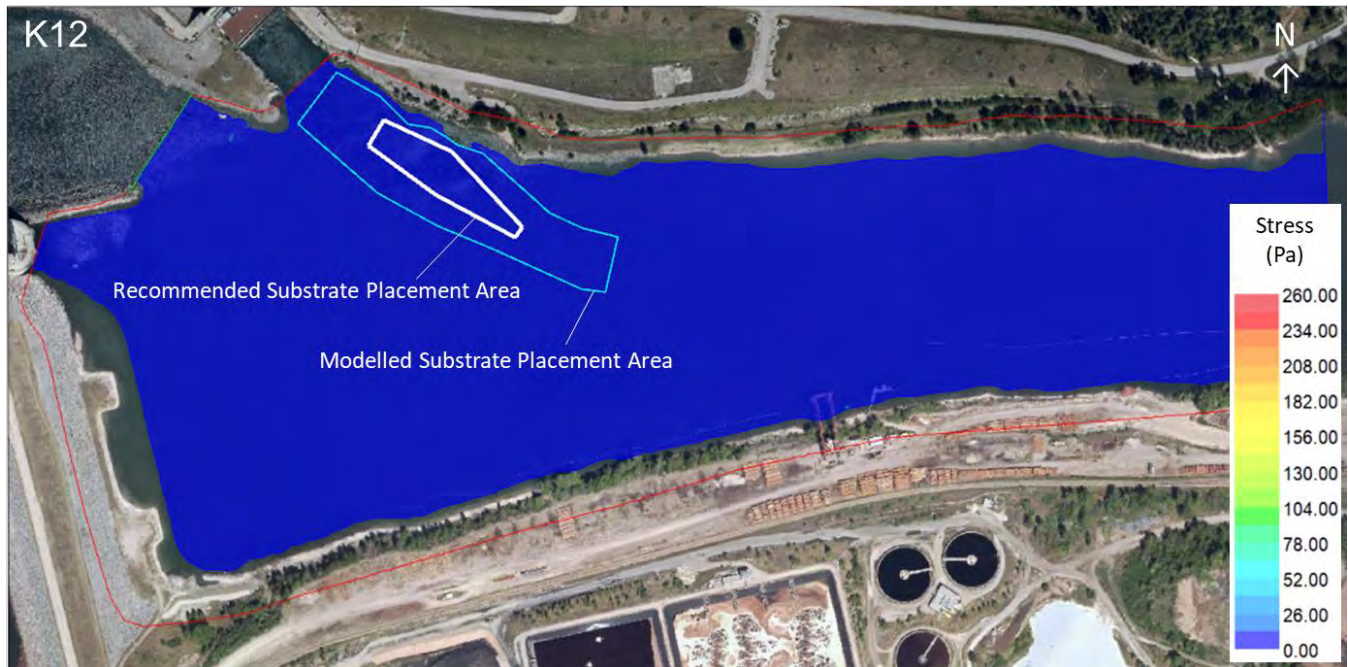
Figure 5: River2D Simulated Shear Stresses (Pa) for the K12 (Fines Deposition) Scenario (Extracted from Hydrodynamic Modelling by Ecofish (2020))
