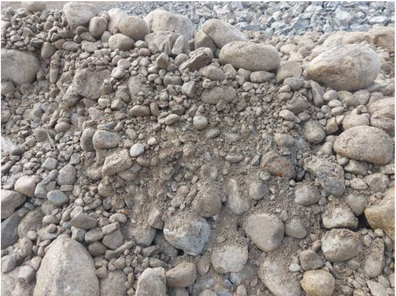
Photo 4: Evidence of fines (< 20 mm) in stockpile. Photograph taken facing SW
