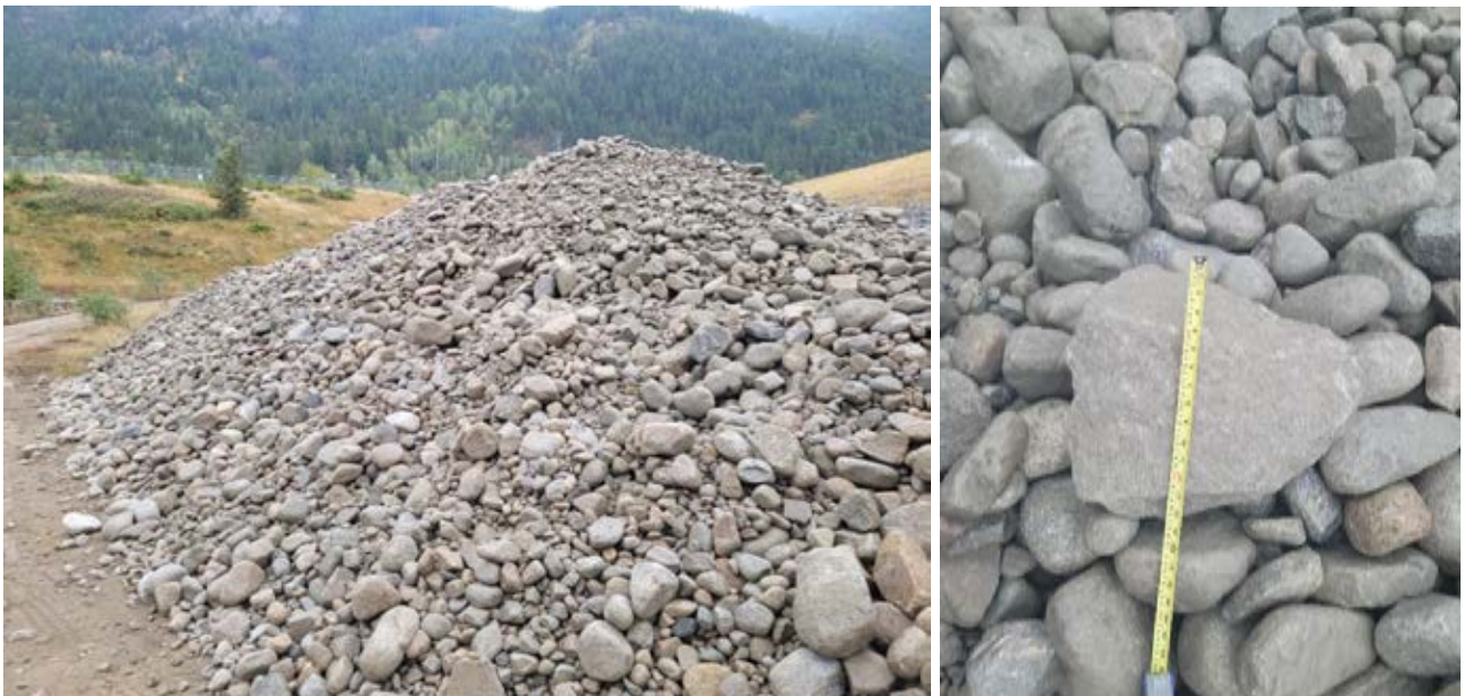
Photo 2: Material stockpile and example of substrate material with excess fines
