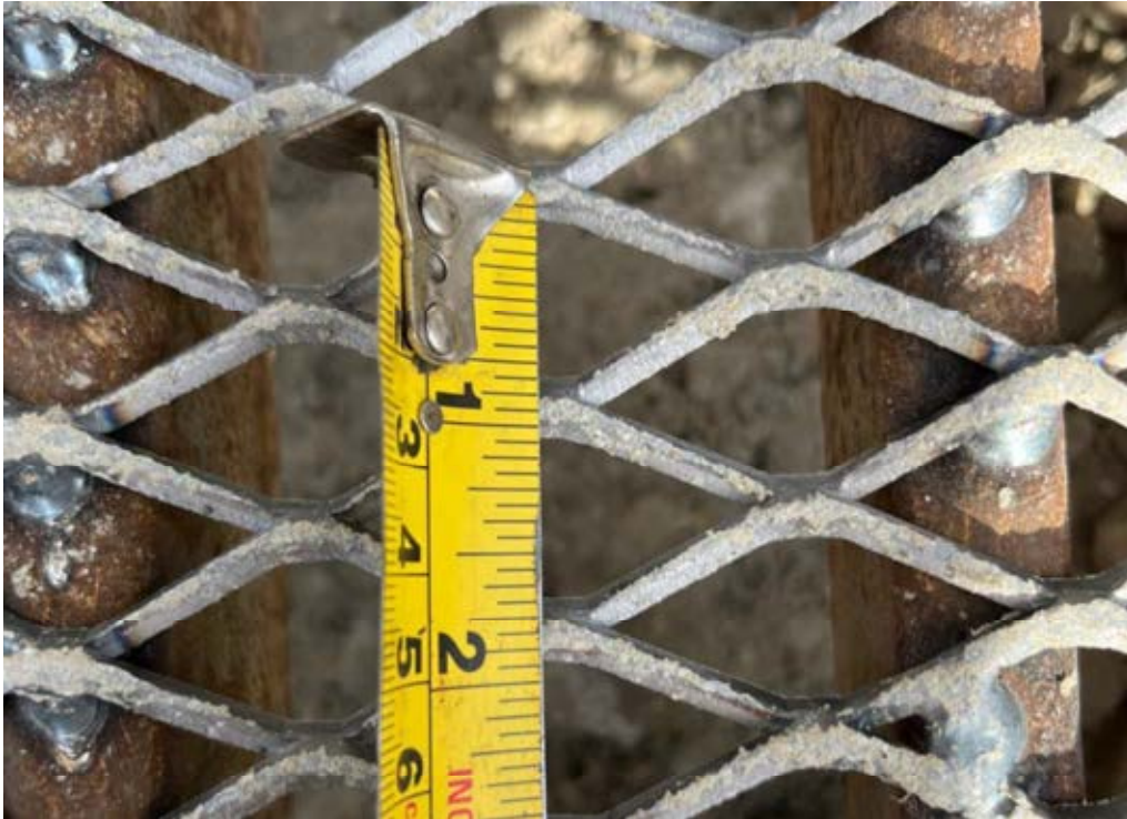
Photo 3: Mesh welded onto bucket with \frac{3}{4} " openings
