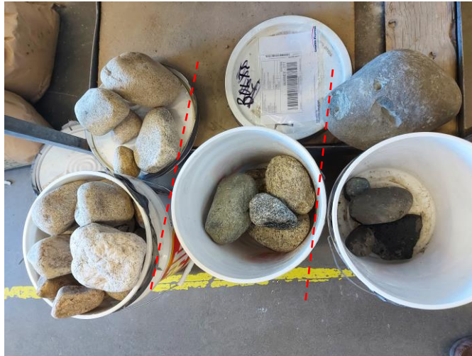
Photo 1 Rock Samples Collected for Testing (sub-sample -S01-S02 to S03, left to right)
