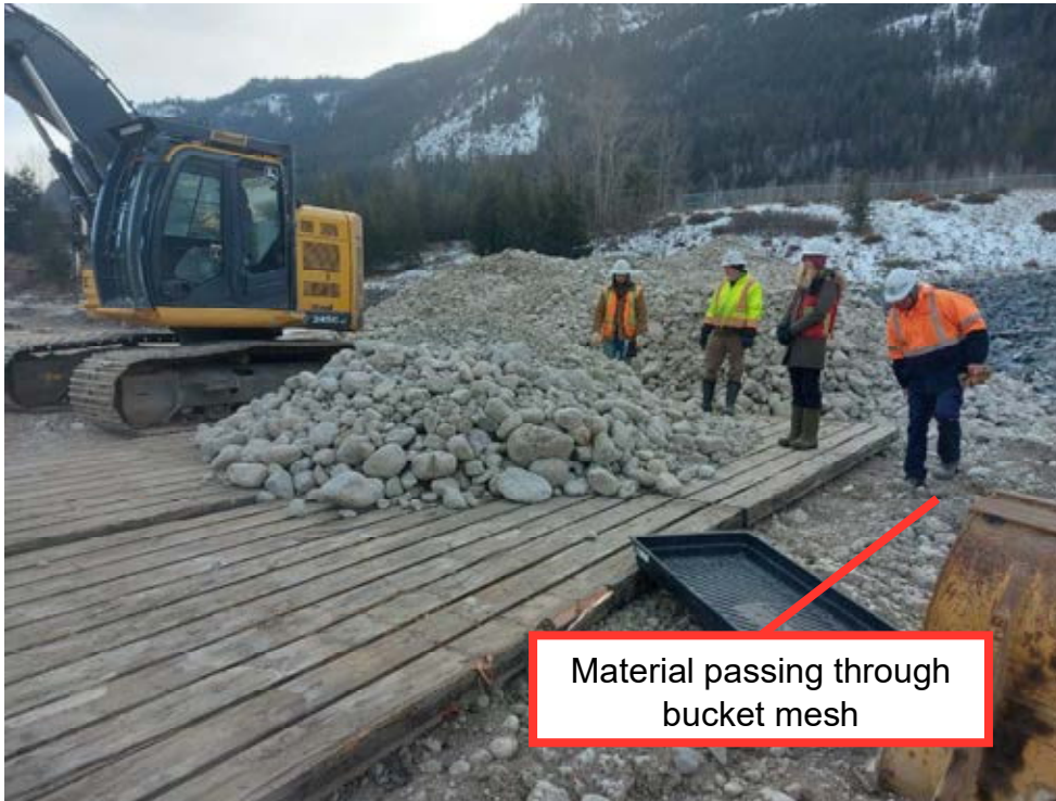
Photo 5: Sieved stockpile and material passing through bucket mesh (deposited sands and fine gravel observed in the soil pile)
