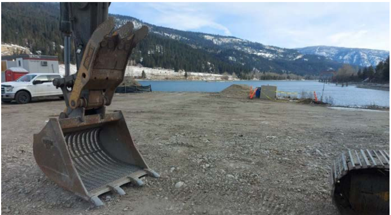
Photo 2: Excavator skeleton bucket with welded mesh
