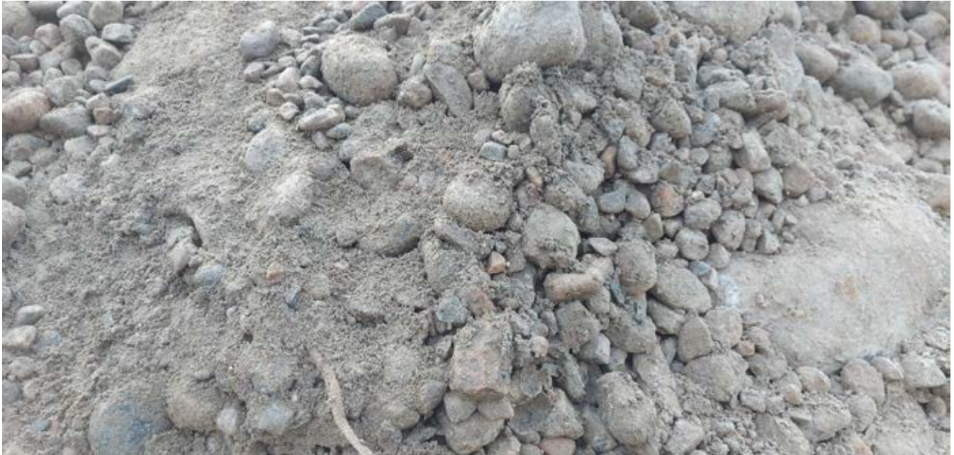
Photo 5: Additional evidence of fines (< 20 mm) in stockpile. Photograph taken facing NW
