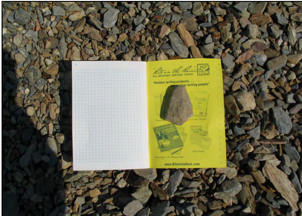
Photo No. 37: Taken on 2007-05-23 at Nixon Creek Close-up view of typical gravel material for the boat launch ramp.
