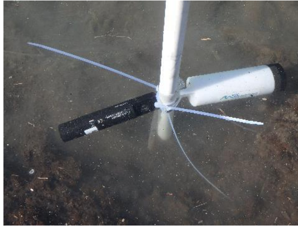
Figure 3-9. Onset conductivity ( \mu\text{S}/\text{cm} ) and PME dissolved oxygen (mg/L) data loggers installed in one of the cleared wetlands at the Bush Causeway North site, May 2016. Both data loggers also logged water temperature ( ^{\circ}\text{C} ).
