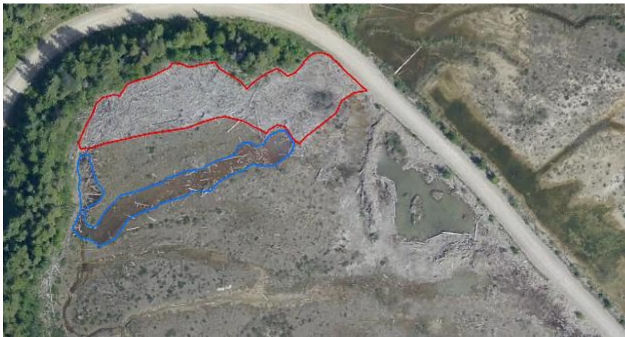
Figure 6-3. Areas that could be cleared of wood debris at the Bush Causeway North site. The red polygon indicates the terrestrial area that could be cleaned and the blue polygon is the wetland that could be cleaned.
