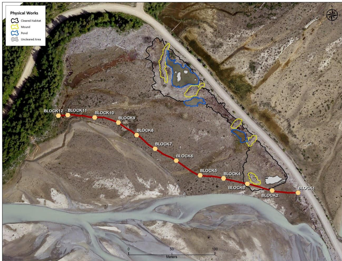
Figure 3-2. Location of log boom and lock blocks installed in June 2016 at the Bush Causeway North physical works site.
