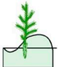
Mound or prepared spot, tree improperly positioned. Code C2
