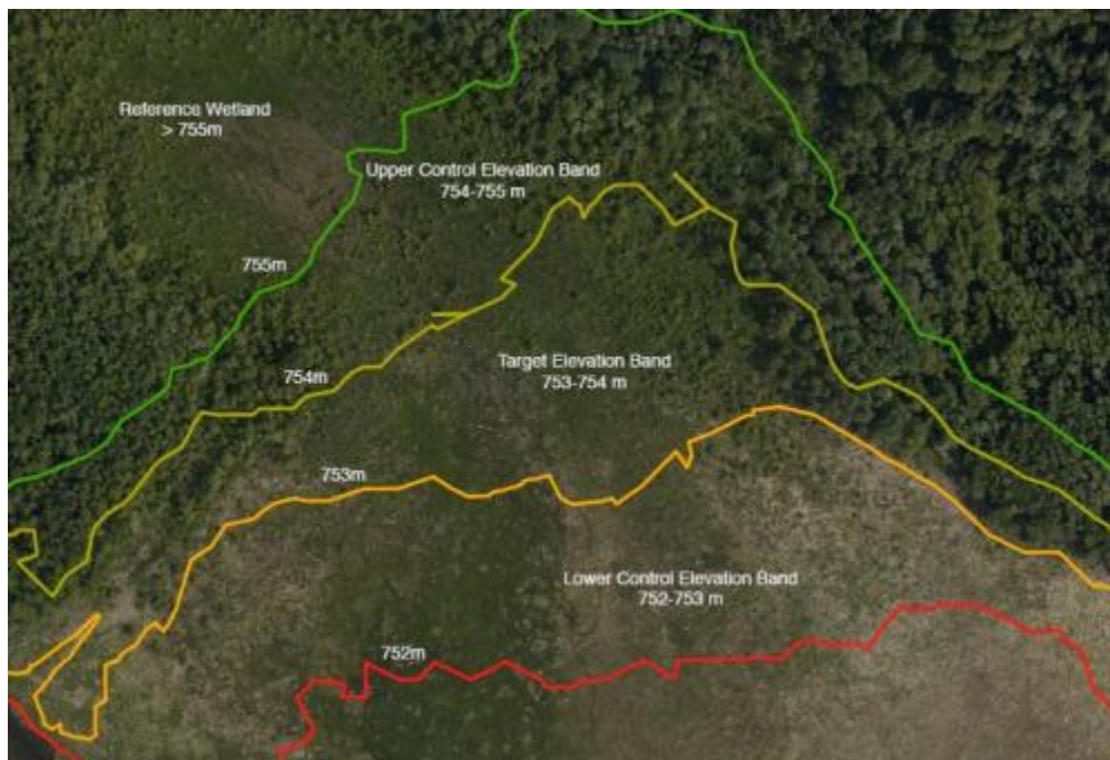
Figure 10-1: Sampling strata of an index monitoring site showing target, control, and reference elevation bands
