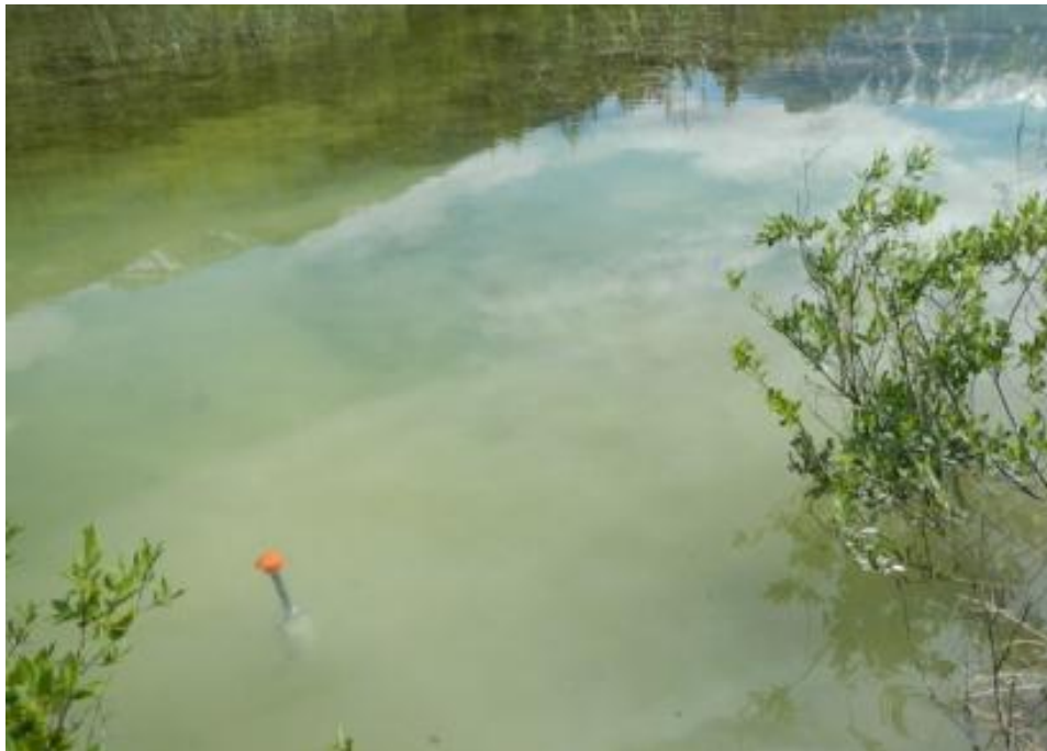
Figure 5-3: Dissolved oxygen and conductivity sondes installed in an aquatic wetland (pond) in Kinbasket Reservoir
