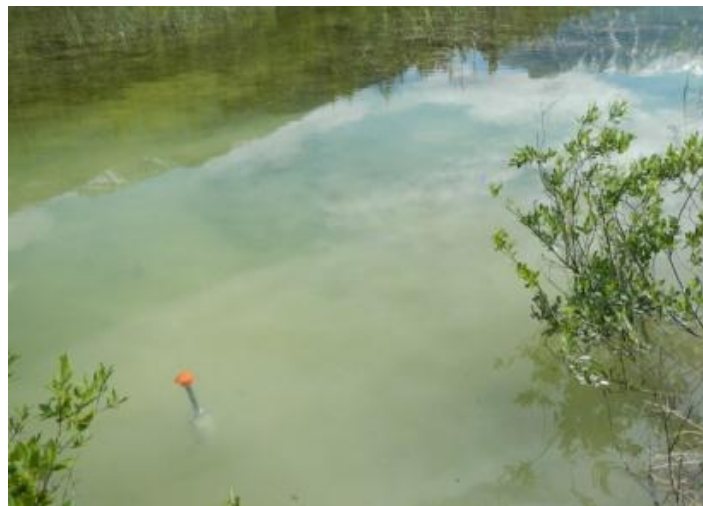
Figure 4-7: Image showing a dissolved oxygen and conductivity datalogger assembly installed in Kinbasket Reservoir
