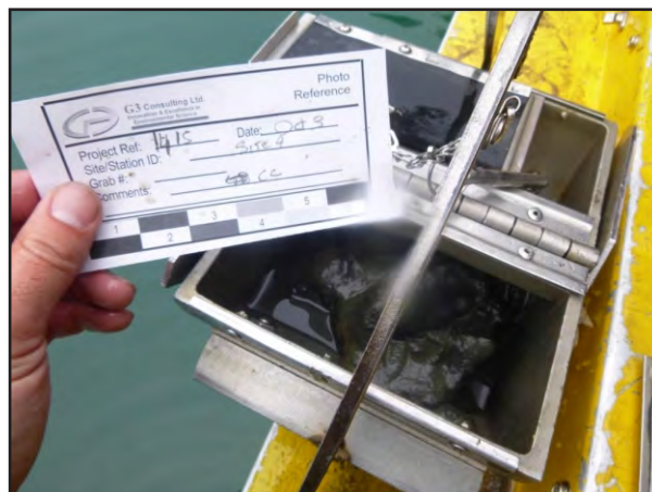
Photo 66: Stainless steel Ponar used for collecting sediment
